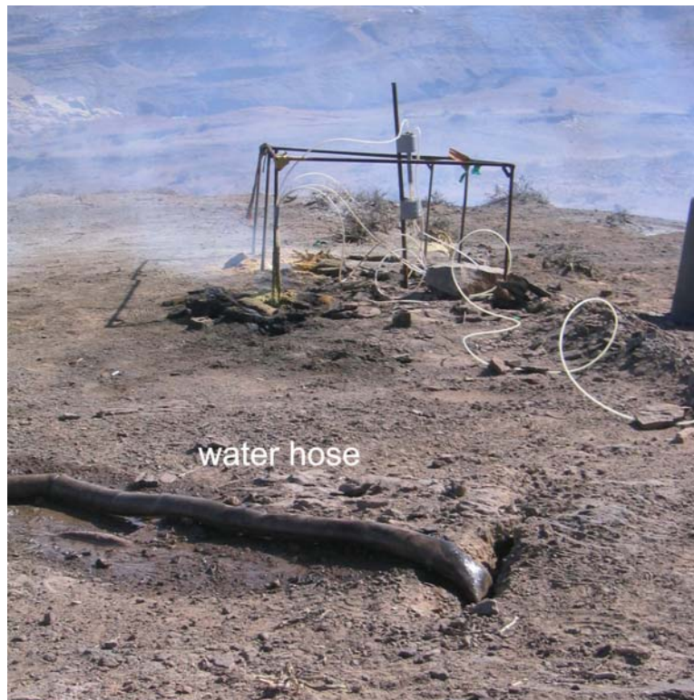
Figure 36: October 23 rd : 2 nd flooding test (about 4.5m 3 water flooding close to the monitoring location 3)
