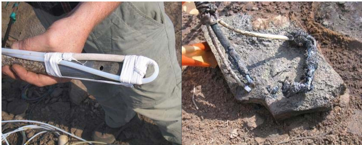
Figure 27: Example of the original membrane as of June 14 th and after removal at October 16 th ; the membrane is considerably fouled with condensates (disconnection between membrane and Teflon tubing occurred as a result of removal from the vent)
