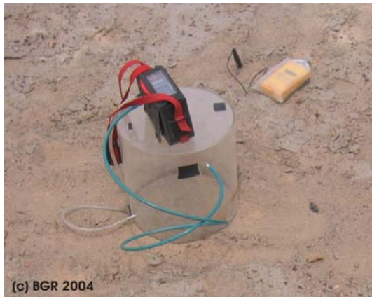
Figure 4: Plexiglas emission chamber with multi-gas instrument Multiwarn II (internal pump circulating the gas) and temperature measurement at fire zone 3_2
