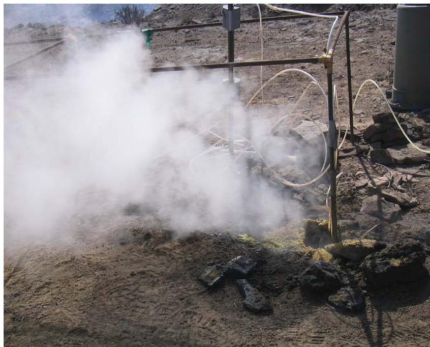
Figure 37: Steam eruption at location TL3.1, shortly after flooding experiment started
