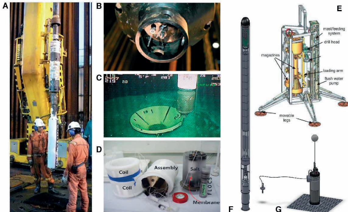
Illustrations of the SmartPlug (A), GeniusPlug (B-D) and MeBo seafloor drill (E) and associated MeBo-CORK components (F, G).
