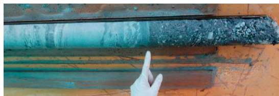
Figure 1: Principal slip surface of the Alpine Fault, identified in a core sample. PSS separates cataclasites from underlying gravel.
