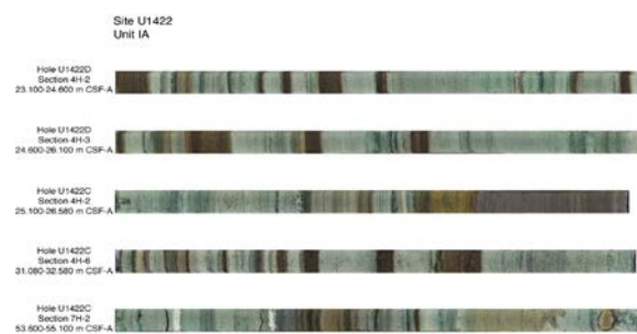
Figure 3. Representative dark and light layers in Lithological Subunit IA, Holes U1422C and U1422D (Expedition 346 Scientists, 2013). Note that the contrast in the core images has been enhanced to highlight sedimentary structures.
