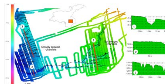
Fig. 2. Multibeam bathymetry map of eastern shelf showing numerous channels on the lake floor. These channels were probably formed during low lake levels when the shelf was subaerially exposed.
