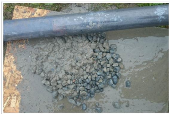
Figure 2: Drillcore from first coring test in gravel (Photo: R. Niederreiter)
