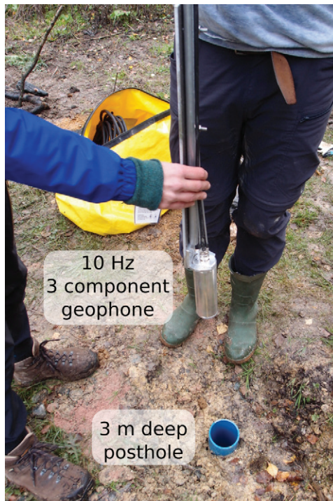
Fig. 1: Installation of 10 Hz geophone in 3 m deep post-hole.
