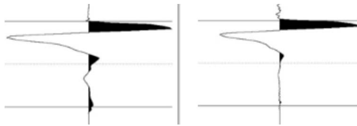
Fig. 5.1.2.1 Extracted wavelet for cruise BalTec (left wiggle). Resulting wavelet after the application of the minimum phase filter (right wiggle).
