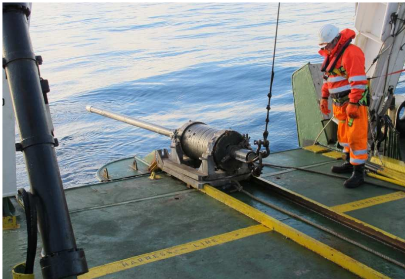
Fig. 61: Gravity corer still mounted to the sledge onboard of OGS Explora before deployment.
