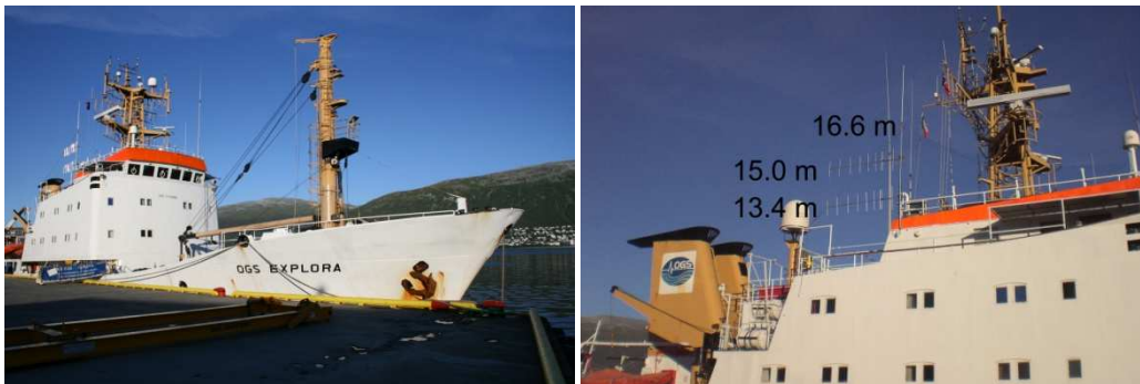
Fig. 40: Sonobuoy antennas mounted on the monkey island of R/V OGS Explora. The height of the three antennas is given in the right picture.
