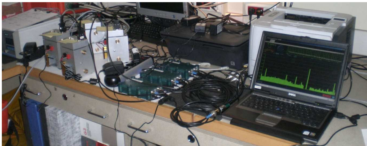
Fig. 41: From right to left: laptop controlling the winradio receivers, 3 winradios (green boxes), four MBS recorders, GPS receiver for time sync.
