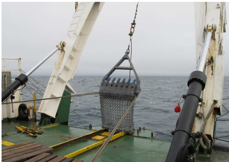
Fig. 63: BGR's chain bag dredge hanging at the A frame of the vessel; ready for deployment. This device was used to sample hard rock outcrops at the sea floor.
