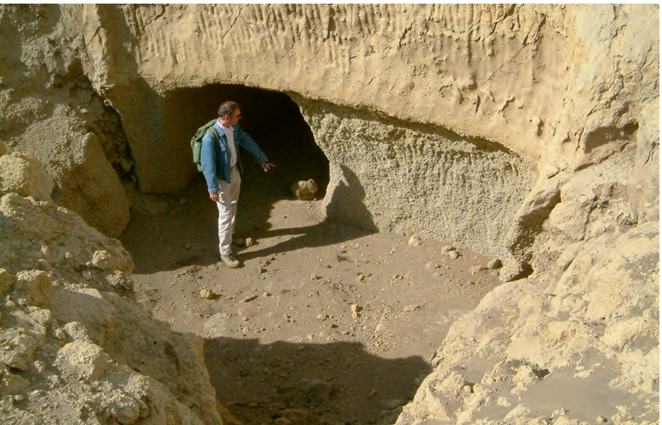
Figure 47: Entrance into adit showing thickness of pumice layer below overburden of tuff west of Mount Meru.
