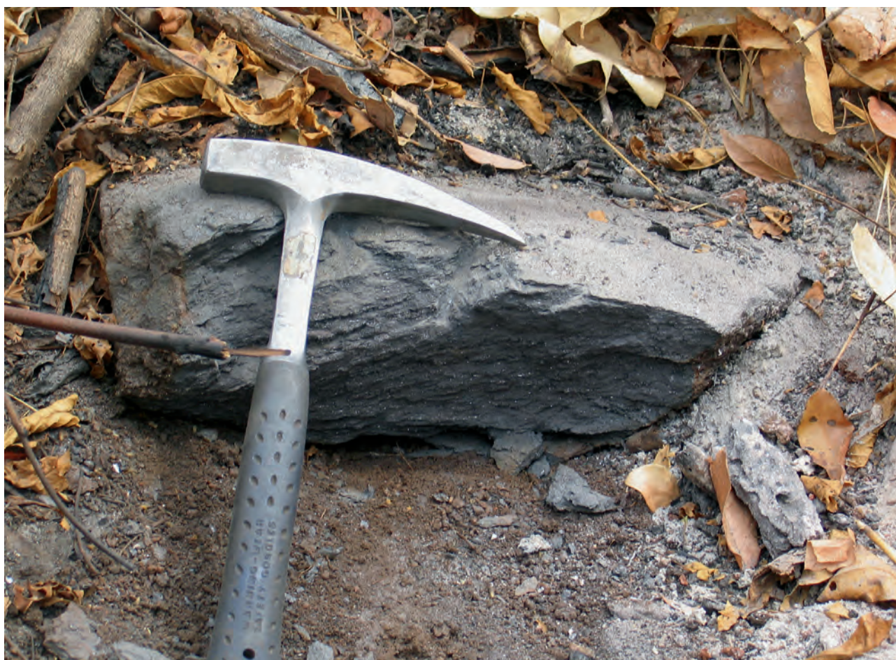
Figure 19: Graphite ore with mixed flake and vein graphite from the Nachingwea deposit.
