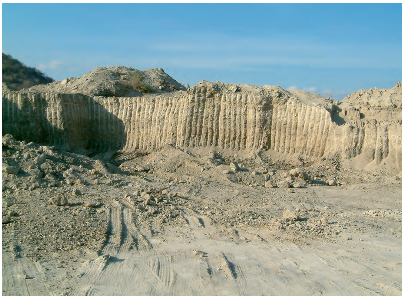
Figure 27: Gypcrete wall in the Msagali open-pit mine.
