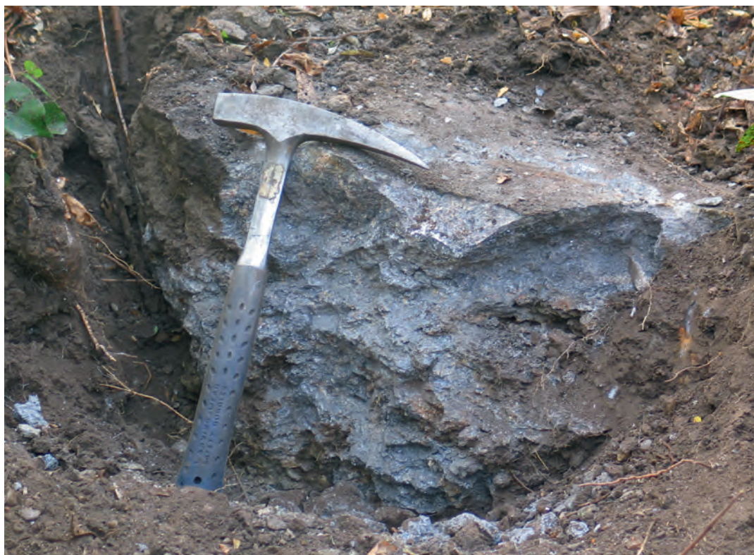
Figure 21: Graphite ore with mixed flake and vein graphite from Mbanga Hill near Ndanda.
