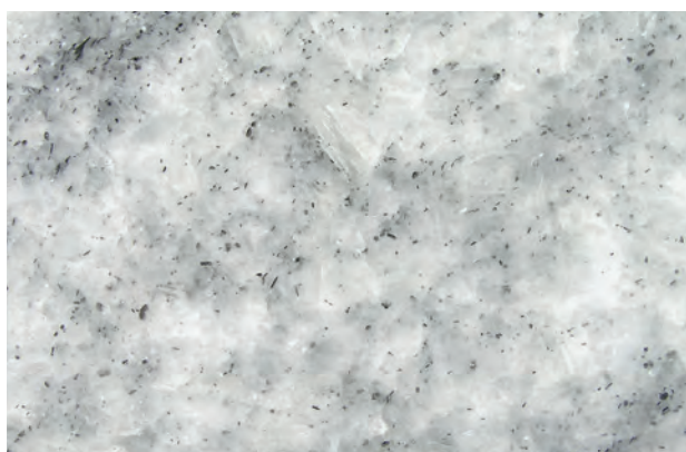
Figure 72: Polished marble with tiny flakes of shiny graphite from the the Nagaga area.
