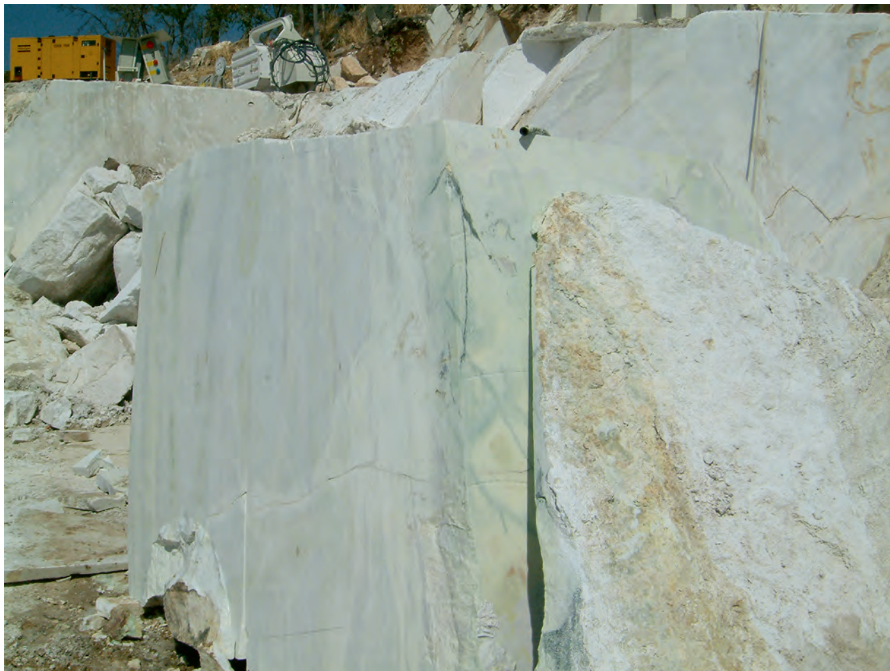
Figure 70: Typical freshly quarried block of white and greenish marble in the Igawa quarry.
