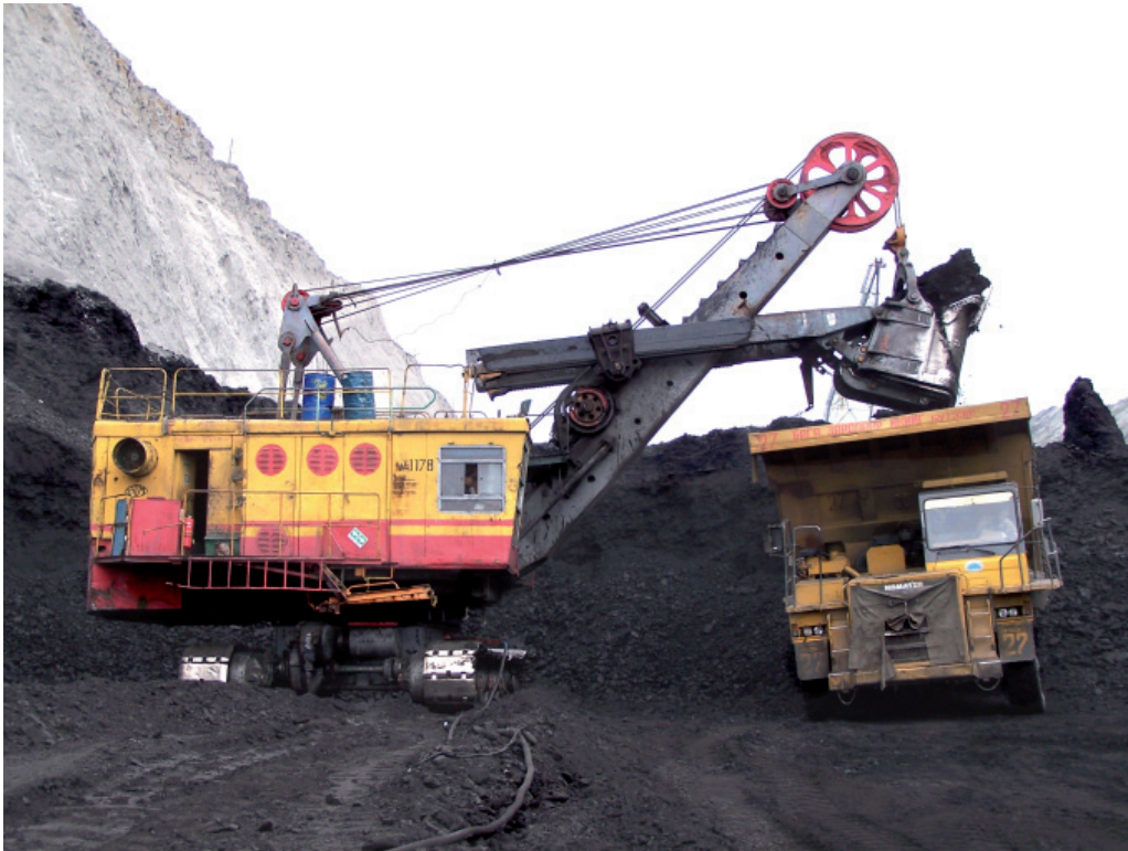
Figure 5.7: Production of hard coal (raw coal) using truck and shovel in the surface mine Baganuur/Mongolia.
