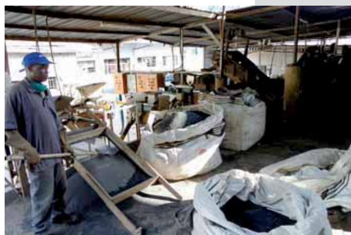
Ore concentrate upgrading at mineral processing plant Gisenyi
