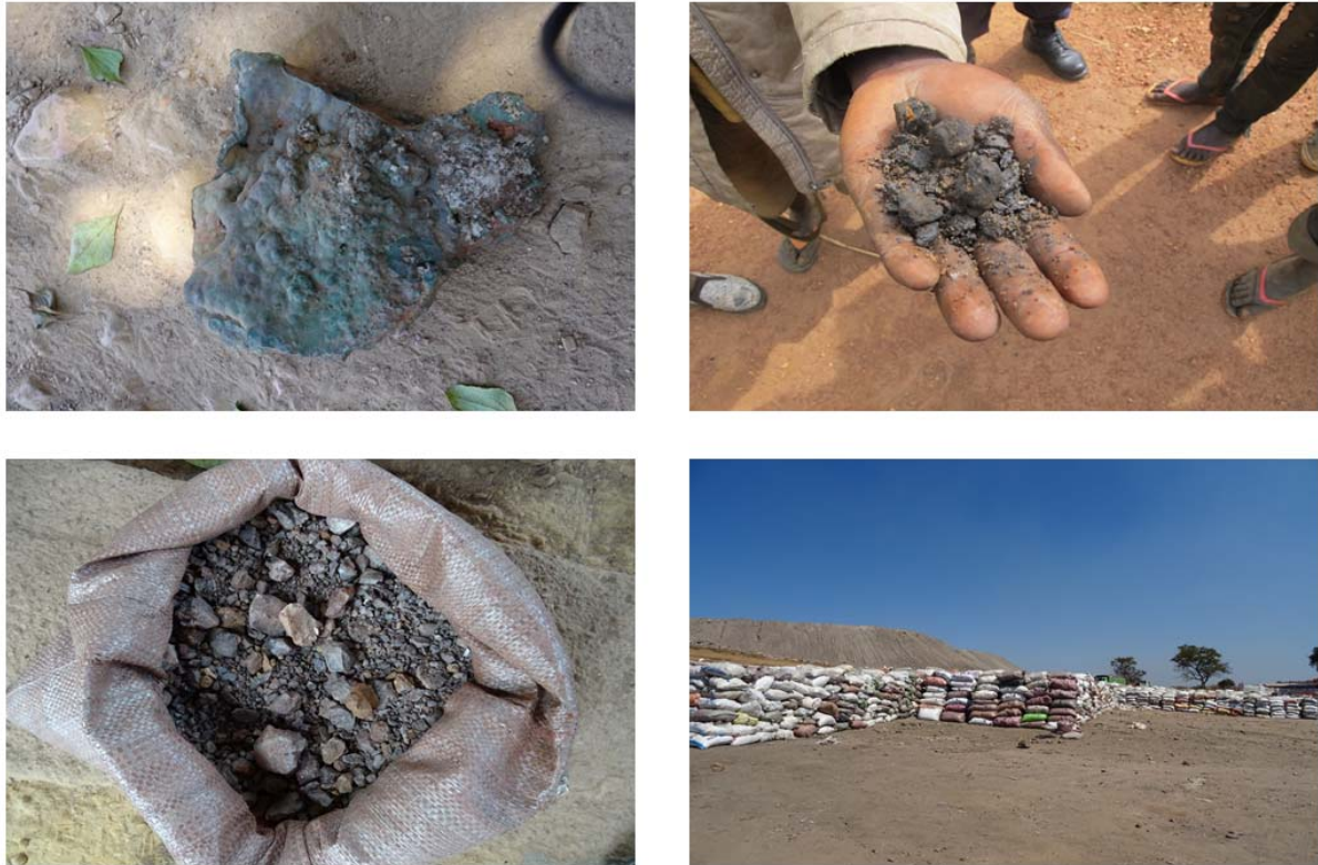
Figure 11 The photographs show typical copper-cobalt ores (copper top left, cobalt top right) which are mined near the surface in small mines and then are filled, partly unsorted or unprocessed, into bags which are stored on the mine until transport.
