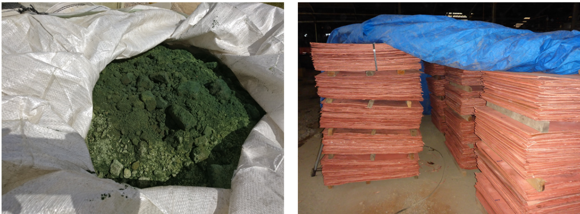
Figure 18 Final products of the intra-Congolese value chain or supply chain. Left cobalt hydroxide, right copper cathodes. These products are manufactured using hydrometallurgical processes that are energy-intensive, require the use of chemicals and technical know-how.
