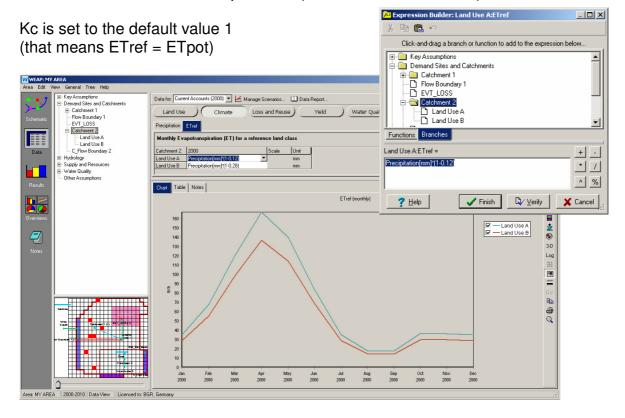
**Surface runoff**: the surface runoff is calculated here as Surface Water Inflow. The runoff coefficient for catchment 2 is 0.16:
