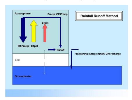
The effective/ ineffective precipitation fraction is a user entry variable as well as the fractioning between surface runoff and groundwater recharge. In our example we will not assign any runoff link from the catchment to the surface water (river), that means all "WEAP-runoff" is groundwater recharge.
