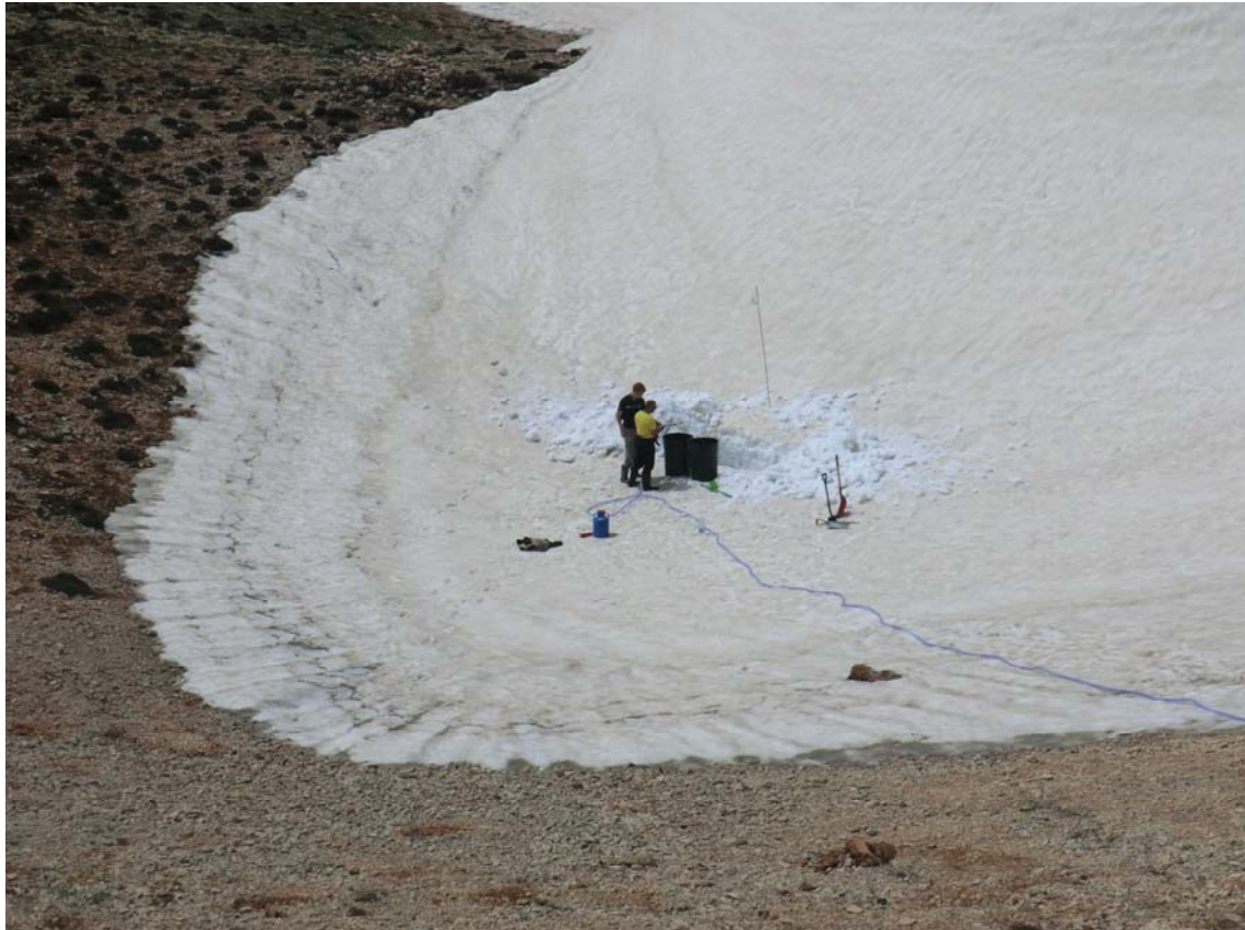
Figure 5: Hole for Tracer Injection near deepest Point of the Doline
