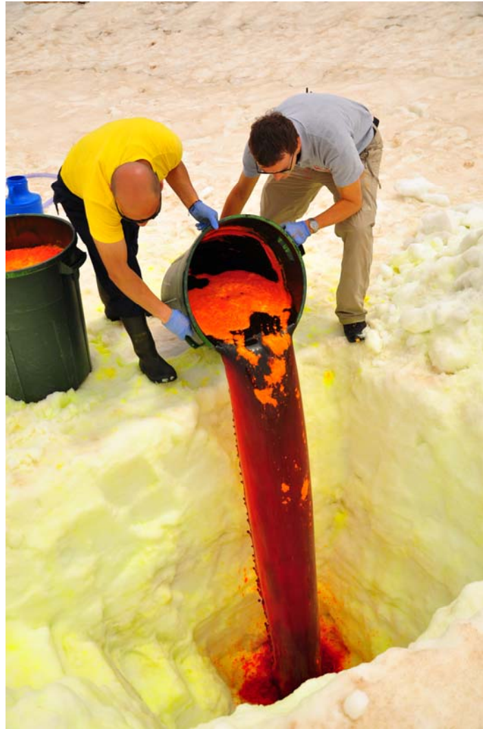
Figure 6: Tracer Injection in Melting Snow
