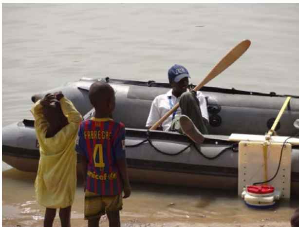
Figure 6 DREM ADCP fixed on a Zodiac boat
