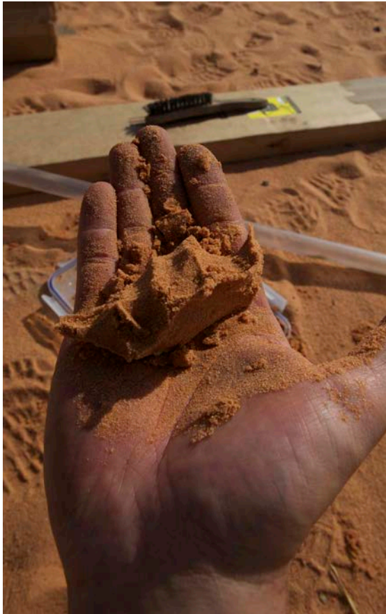
Retrieval of moist sand samples (from 3 to 14m deep in the unsaturated zone)
