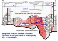
Fig. EW-schematic section to explain controlling processes in the CHC-plume of Hannover-
