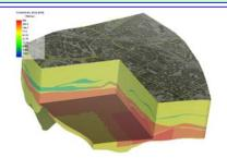
Fig. Subsurface model of the unconfined aquifer of glacio-fluviatile origin (gravel, sand, silt-beds)
