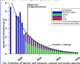
Fig. Prediction of Nat-Att. with transport, reaction and kinetic desorption from coal till 2030 for mass of diss. TCE, cDCE and VC (source: 2)M & P)
