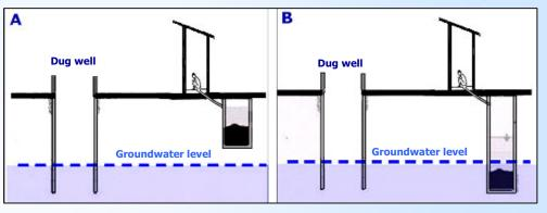
Fig. 2: Latrine pit above (A) and below (B) the groundwater level
