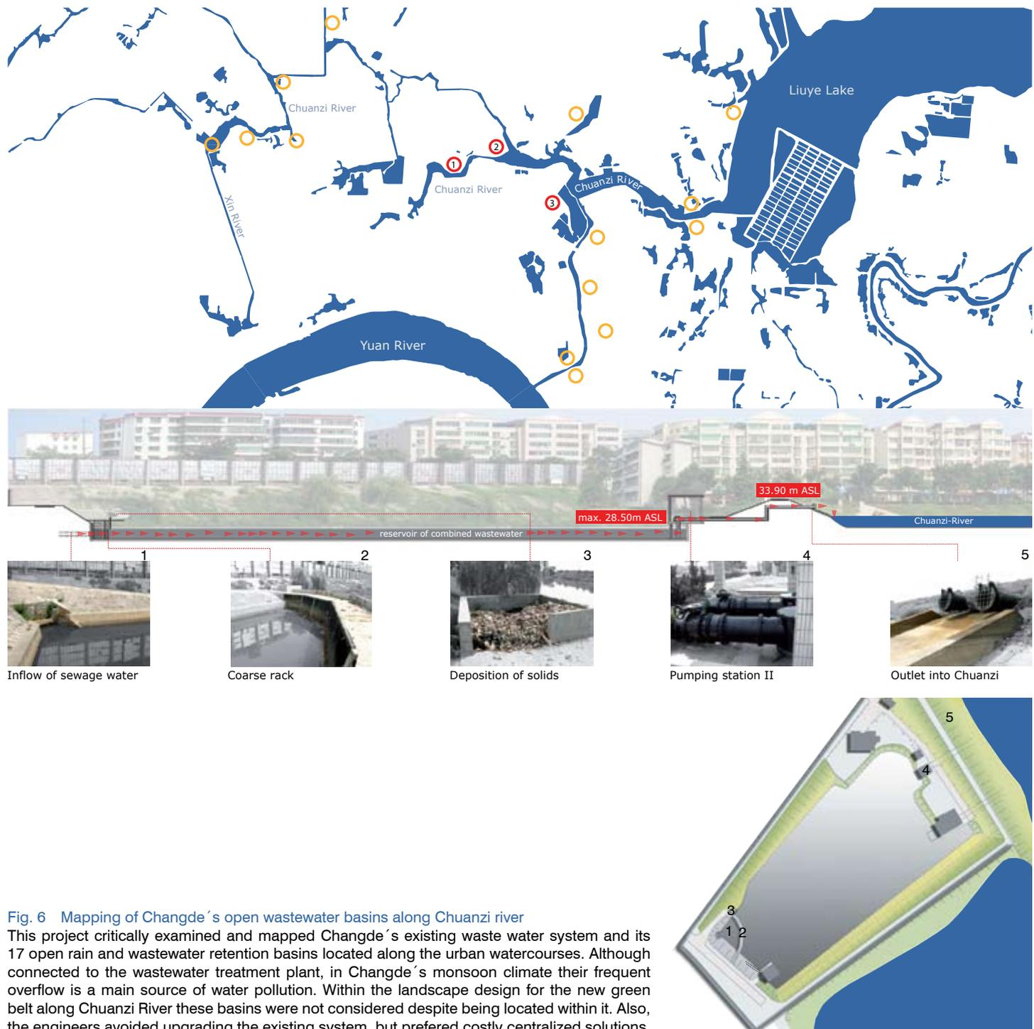
**Fig. 6 Mapping of Changde's open wastewater basins along Chuanzi river**
