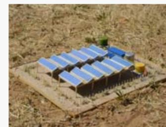
Model of solar thermal desalination plant
