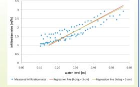
Figure 2: Measured infiltration rates and related water levels at the basin [Zemann, 2008]
