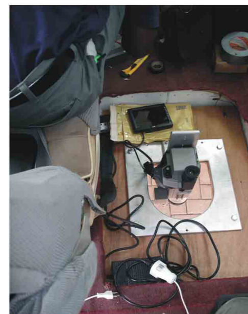
▲ Fig. 3 FLIR ThermoCam PM695 mounted on aircraft PIPER NAVAJO
