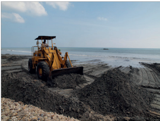
Figure 42: Beach mining of HM at Pulmoddai. Photo courtesy of Lanka Mineral Sands Ltd.
