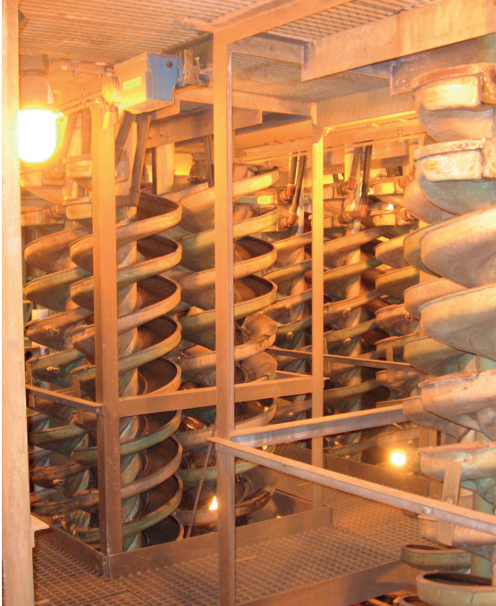
Figure 11: Spirals in the Empangeni MSP of KZN Sands, Republic of South Africa. Photo: DERA.
