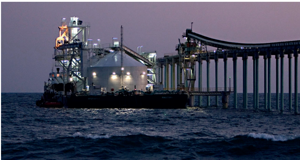
Figure 34: Ship loader at the end of the jetty at Moma, Mozambique. Photo courtesy of Kenmare Resources plc.
