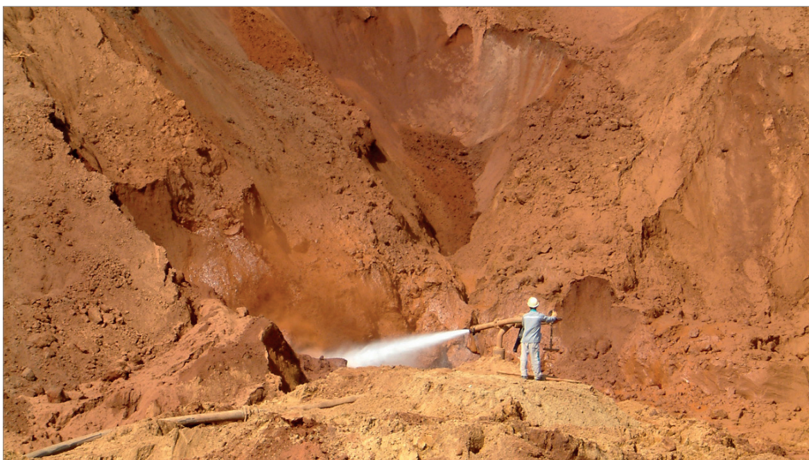
Figure 39: Hydraulic mining of HM rich sands at KZN Sands in KwaZulu-Natal, Republic of South Africa. Photo: DERA.
