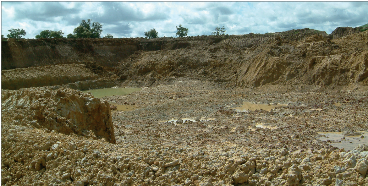
Figure 24: Pit with slime-rich HM sands mined by Doral Mineral Sands in Western Australia, Photo: DERA.
