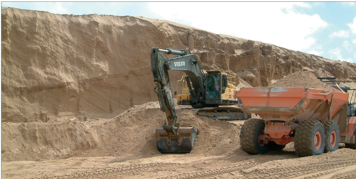
Figure 25: Easy mining of garnet-rich fossil dune sands by GMA Garnet at Port Gregory, Western Australia. Photo: DERA.
