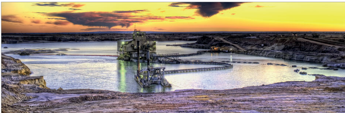
Figure 22: HM dredge and wet concentration plant (concentrator) at Cooljarloo, Western Australia. Photo courtesy of Tronox Ltd.
