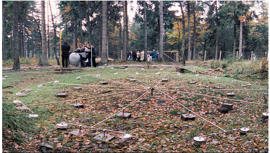
Wind-noise-reducing pipe array, which functions as a filter to remove background noise from the infrasound signals.
