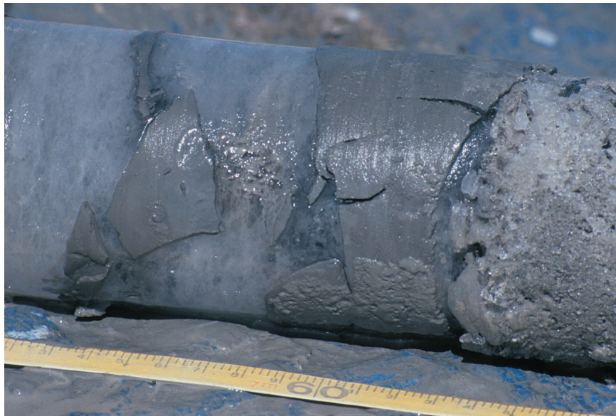
Borehole core from a frost mound; marine clay is fragmented by ice.
