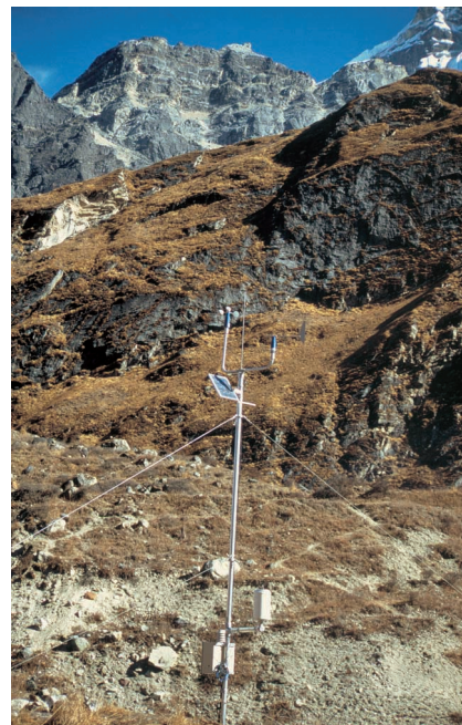
Automatic gauging and meteorological stations, monitoring the rate of flow in the outlet stream and recording weather data.
