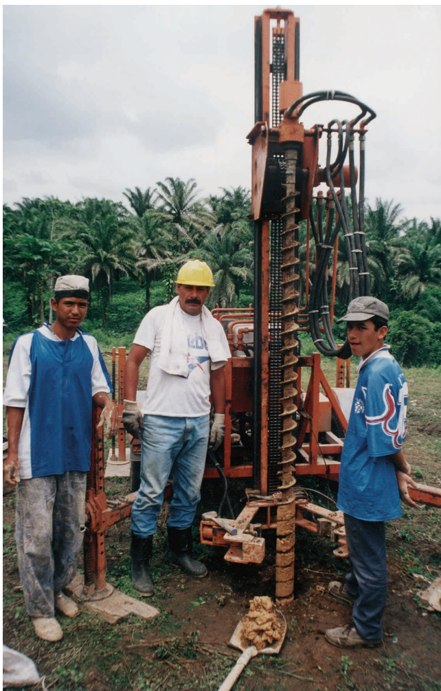
Drilling in allophane-bearing eluvial loam in Pichincha province in Ecuador.
