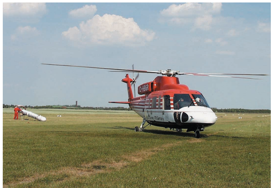
BGR helicopter and „bird“ preparing to start a survey flight.
