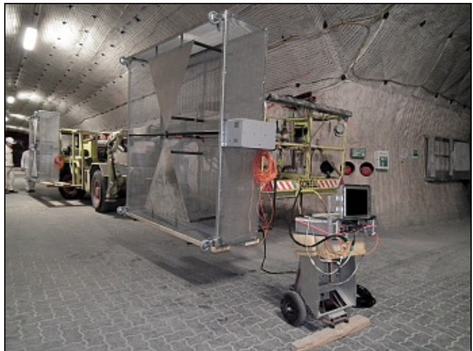
Shielded 40-MHz antennas on a transport vehicle with a recording unit.
