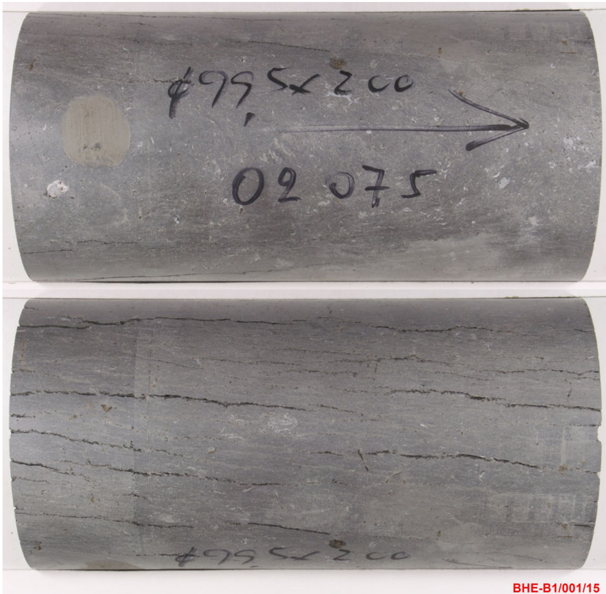
Fig. 15 The BHE-B1/001/15 sample used in the complex strength test. Some shrinkage cracks parallel to the bedding indicate desiccation of the material.
