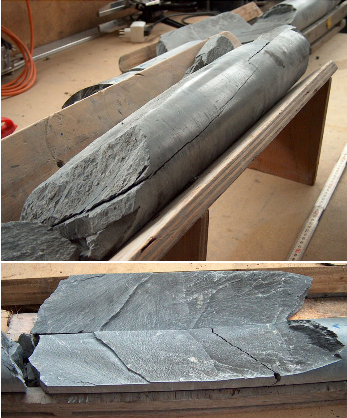
Fig. 2 Core from BLT-17 showing freshly formed axial fractures. There is neither a slickenside (which would indicate a tectonic fault) nor any trace of gypsum crystals (which generate within a few days in any crack opened in the EDZ due to the impact of atmospheric oxygen) on the interface.
