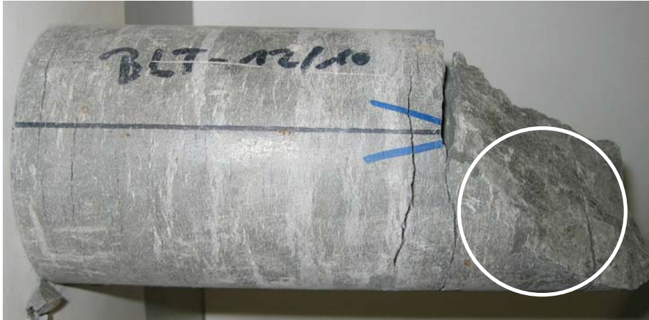
Fig. 3.2: Cylindric sample (BLT 12/10) after mechanical testing. Samples for mineralogical and optical investigations were taken from the labeled area.
