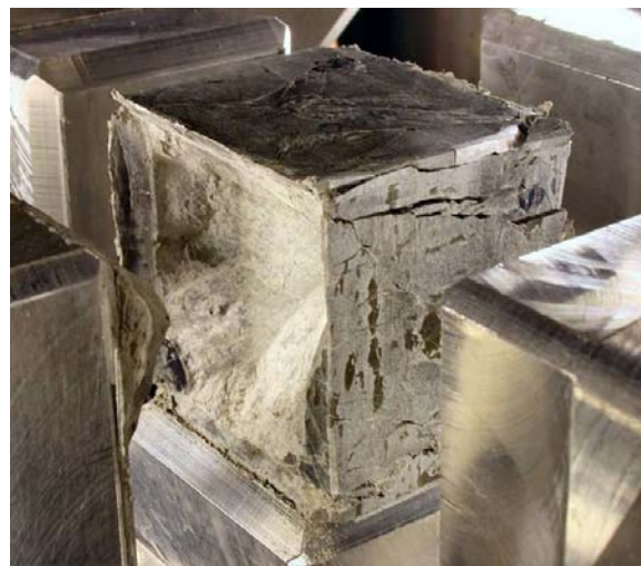
Fig. 38 Cubic Opalinus Clay specimen after true triaxial compression test.
