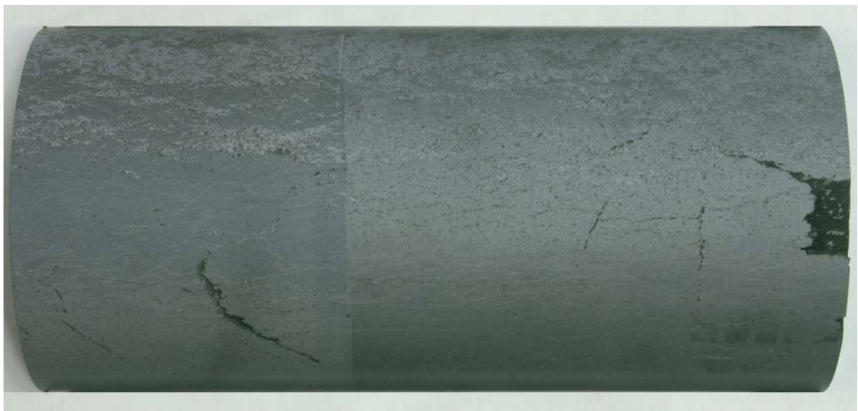
Fig. 6 A breakout at the edge of a specimen generated during trimming on a lathe (p-sample 08018 from BLT 14).
