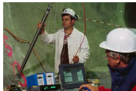
Permeability measurements characterise the disturbed zone
