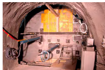
The niche shown on the left was permanently monitored for 10 years after backfilling
