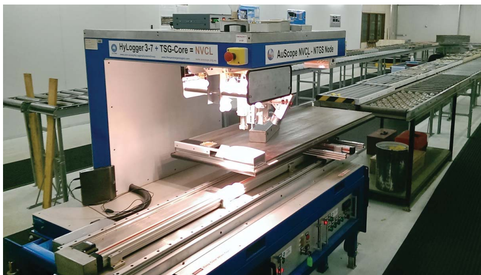
Figure 1. One of the NVCL HyLogger-3 instruments. The spectrometers and control electronics are embedded in top section of the blue frame. Below that, the lighting system directs the illumination onto the calibration block at the beginning of the X–Y translation table. The data-acquisition system, X–Y table controller and power supply unit are in the blue frame under the X–Y table.
