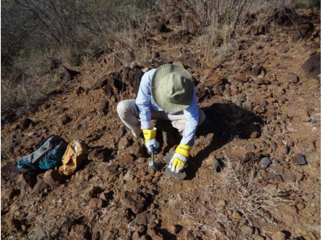
Figure 53: Preparation of a fresh and unaltered rock of sample PK7 (E 194461/ N 102517) suitable for ^{40}\text{Ar}/^{39}\text{Ar} age dating on 27/02/2014.
