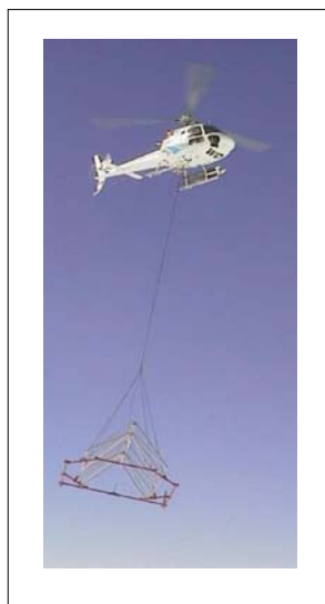
Helicopter with the antenna rig
