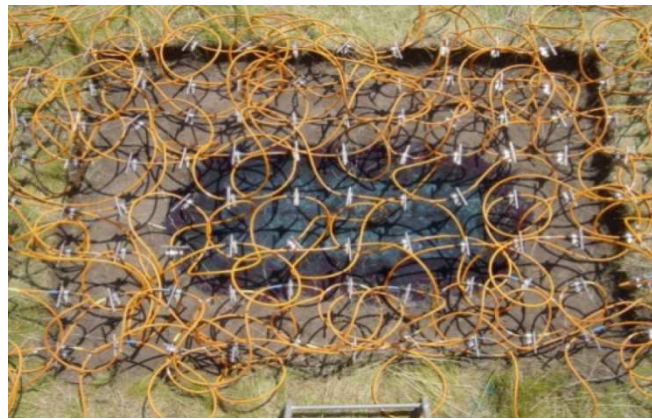
➤ 4D – electrical resistivity tomography (ERT) during infiltration experiment with a brilliant blue tracer
