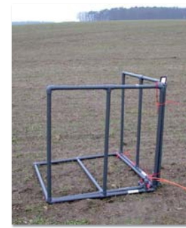
Figure 1: Small handy loops for MRS noise measurements (Standard equipment of MRS MIDI, Radic Research)
