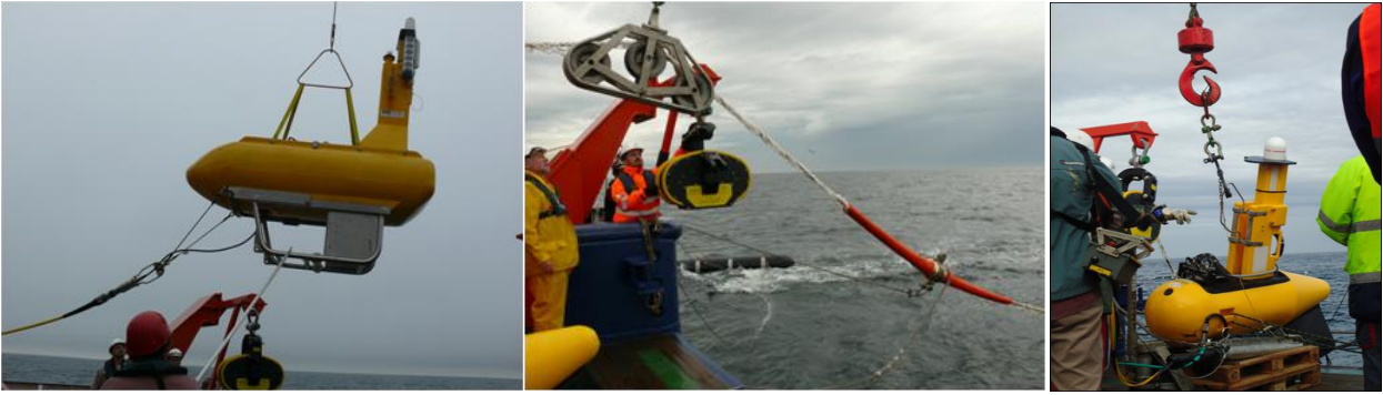
Fig. 5.1.2 Streamer end buoy with GPS (left), bend protector with connecting rope to the paravan; also visible Fairlead block and multi wheel block for streamer deployment (middle), GI gun float with GPS (right)
