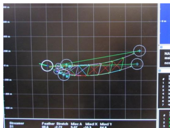
Fig. 5.1.3.1: Spectra navigation system with the screens for QC of sensor data (left), navigation window (2 nd left), binning control (2 nd right), and QC of streamer positions (right)
