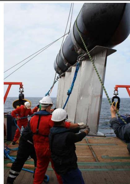
Fig. 4.1 Deck handling of paravane
