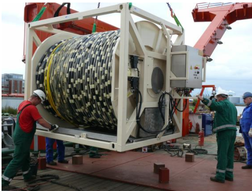
Fig. 5.1.3 Special constructions for proper operation the 3D seismic onboard components. Foundation for streamer winches (installation of winch) – (upper left), support frame for Fairlead block (A) and auxiliary arm assembly for umbilical (B) – (upper right), welded boss (A) for mounting a block for the trawling door rope; also visible block (B) with rope for GI gun deflection
