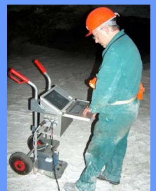
Mobile data recording unit with operator at measurements in a drift in salt.
