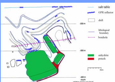
Vertical geological section in a salt mine with results from radar measurements in a horizontal borehole.
