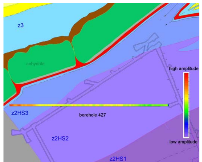
Figure 6. Plan view to a horizontal borehole in salt at the 840 m level with colour coded amplitudes (linear scale) of the direct wave signal
