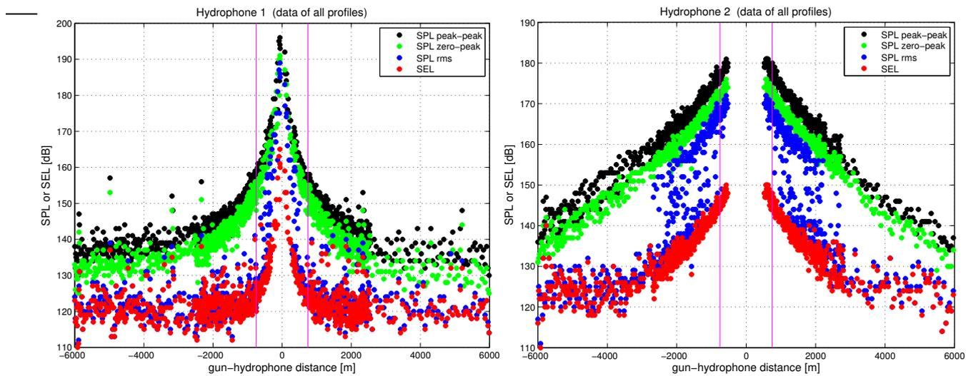
**Fig. 3.4.1-10:** Overview figure with  $SPL_{\text{peak-peak}}$  (black),  $SPL_{\text{zero-peak}}$  (green),  $SPL_{\text{rms}}$  (blue) and SEL (red) measured for all shots along all profiles for the upper (left panel) and lower (right panel) hydrophone. Vertical lines are at 750 m.
