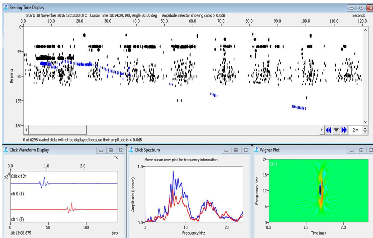
**Fig. 3.4.4-3:** PAMGuard screenshots of Acoustic Detection 501. LF Click detector display showing delphinid click train, click waveform, spectrum and Wigner plot.
