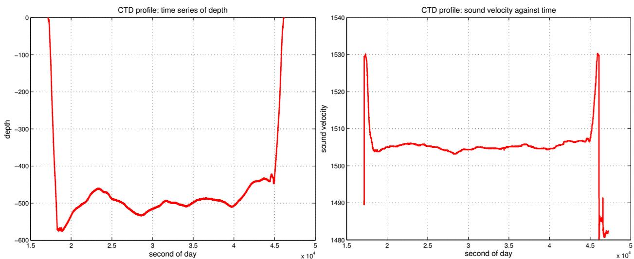
**Fig. 3.4.1-2:** CTD depth (left panel) during the GI-gun calibration varies approximately between 450 and 550 m.
