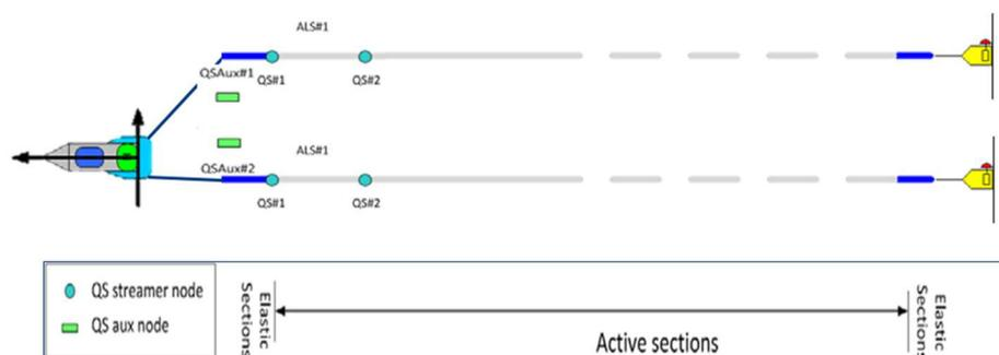
**Fig. 3.4.4-4:** Layout of QuietSea in-water modules with the 4 high-frequency QS#1, QS#2 in each streamer and QSAux#1, QSAux#2 at each source (low frequency detections from 12 channels of each streamer)
