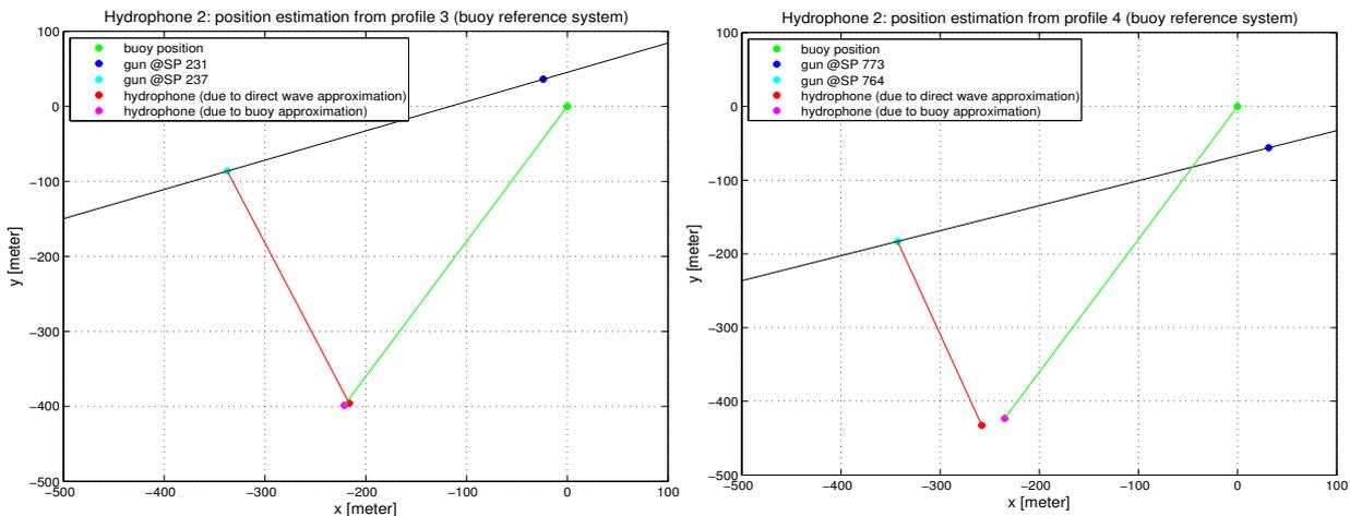
**Fig. 3.4.1-5:** Estimation of the deep hydrophone position due to the minimum direct wave approximation (red dot) and due to the buoy approximation (pink dot). Differences are only 5 m for profile 3 (left panel) and 25 m for profile 4 (right panel). Shot point spacing is 50 m, therefore 25 m is the corresponding error for the hydrophone position.
