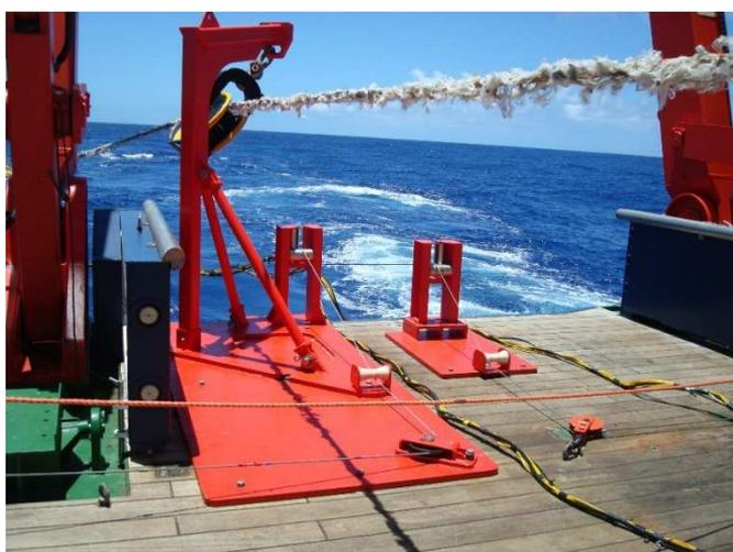
**Fig. 3.4.2.1-2:** Support frame for fairlead block and the two auxiliary arm assemblies at the stern bulwark for the GI gun umbilicals. etup of seismic streamers and sources during 3D data acquisition.
