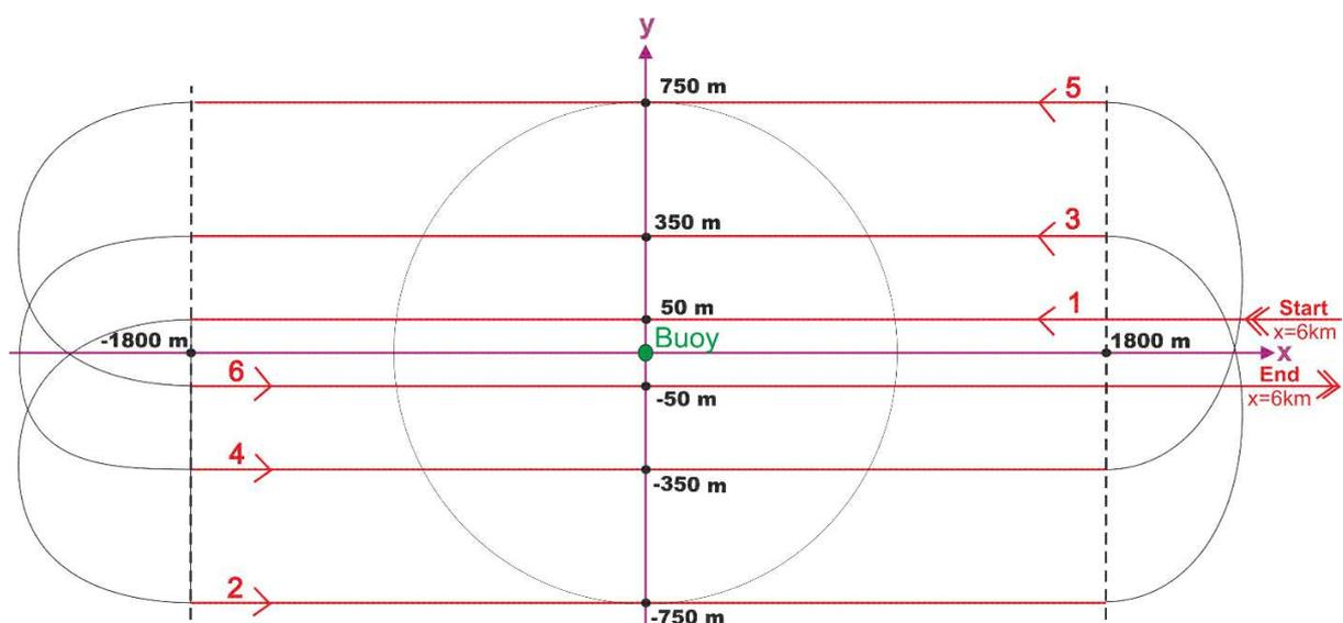
**Fig. 3.4.1-6:** Profile plan for the GI-gun calibration. The buoy shall be passed by six profiles providing different distances and azimuths for each shot point. The profile direction is oriented in the buoy drift direction.
