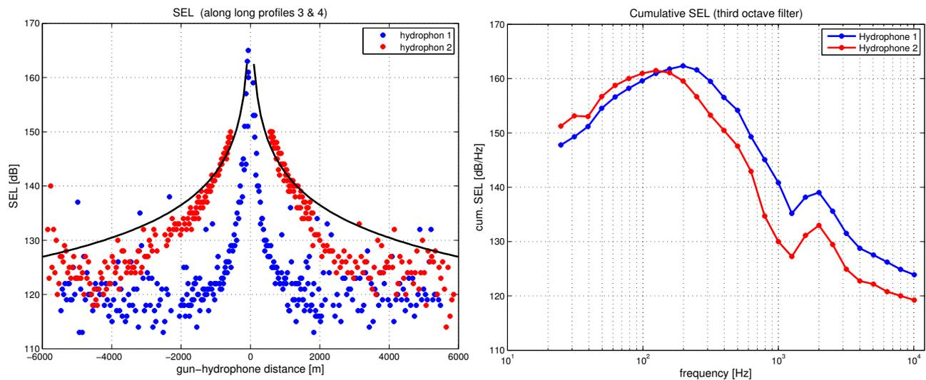
**Fig. 3.4.1-11:** Both long profiles 3 & 4 combined yield SEL in the left panel. A spherical decay with 145 dB re 1  $\mu\text{Pa}^2\text{s}$  at 750 m is illustrated by the black line.  $SEL_{\text{cum}}$  (right panel) adding all shot energies peaks at 200 Hz for the shallow hydrophone, for the deep hydrophone dispersion is already visible by damping higher frequencies.
