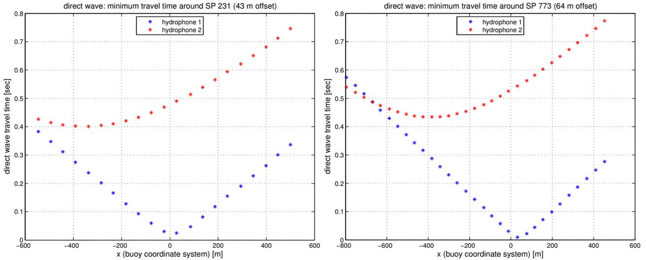
**Fig. 3.4.1-4:** Travel time of the direct wave measured by the upper (blue) and lower hydrophone (red) for shot points along profile 3 and 4 (left and right panel). The hydrophone is located perpendicular to the profile at the shot point with minimum travel time in a distance obtained by travel time, sound velocity and depth indicated by the CTD.
