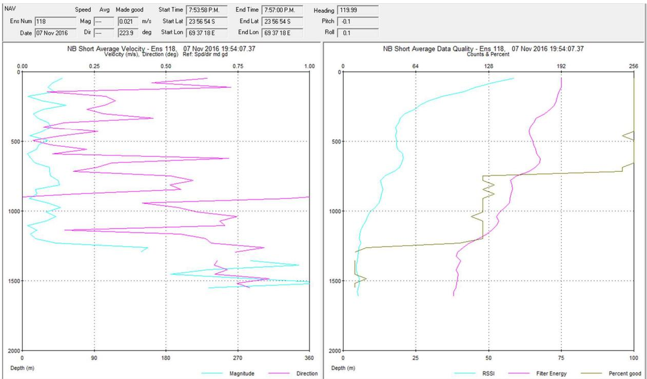
**Fig. 3.4.3.1-3:** ADCP profile in the low frequency range measured on the deployment position of OBS13 (Station 7).
