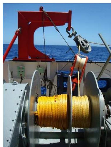
**Fig. 3.4.2.1-3:** Support frame on top of the starboard railing with block for deflecting the towing rope which is winded at the mooring winch.
