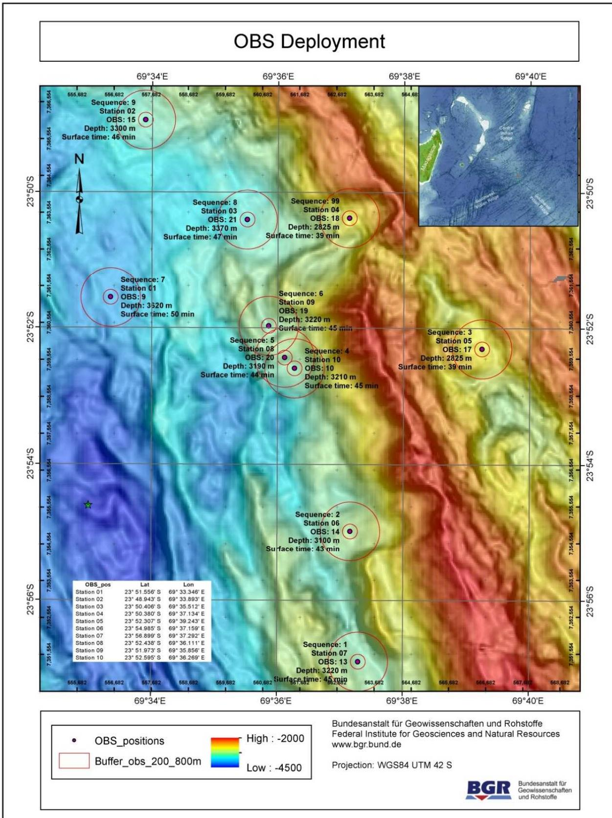
Fig. 3.4.3.1-4: Deployment plan of OBS stations. OBS deployment at station #4 was skipped due to a failed recorder during the setup.
