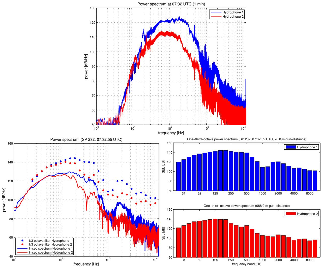
**Fig. 3.4.1-13:** Upper panel: power spectrum of one minute (7.32 UTC, time series in Fig. 3.8) including three shots. Lower panel: power spectrum of at a single shot point: multitaper spectrum of a one-second interval (lower left panel) and one third octave filter applied (lower right panel). The power level depends on the window length of the time series and on the frequency width of the spectral estimate.
