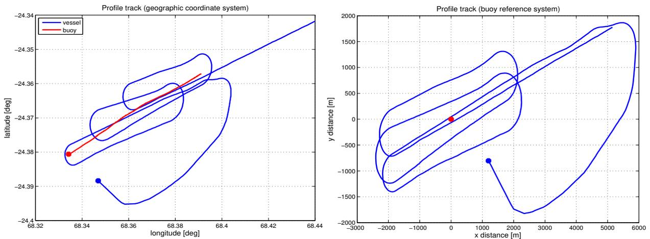
**Fig. 3.4.1-7:** Profile track of buoy (red) and vessel (blue) in geographic coordinates (left panel) and in the buoy reference system (right panel). The latter nicely follows the profile plan of Fig. 3.4.1-6 in spite of significant wind and water currents.
