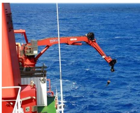
Fig. 3.4.4-1: PAM array cable deployment
