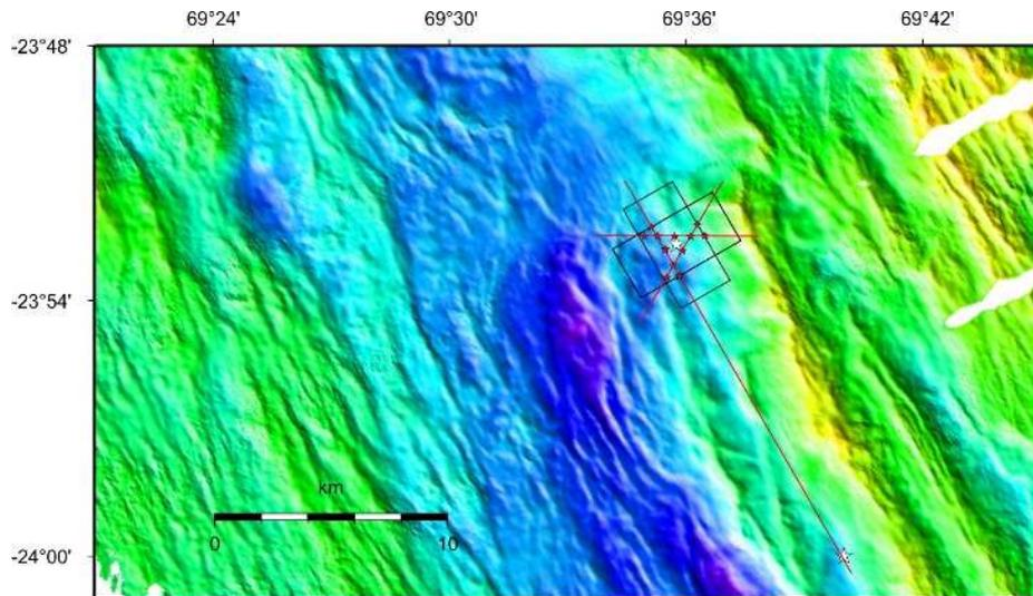
**Fig. 3.1-1:** Bathymetric map of license cluster #4. The white star marks the location of the Edmond Hydrothermal vent field. Black boxes show the orientation of the planned 3D seismic survey areas and red stars mark the proposed deployment positions of the Ocean Bottom Seismometers (OBS).
