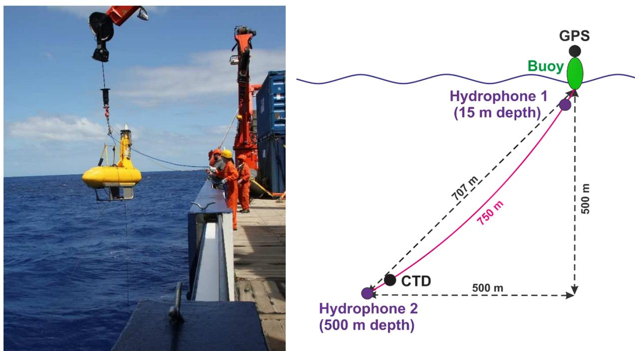
**Fig. 3.4.1-3:** Deployment of the free floating buoy carrying two hydrophones and a CTD below. Due to wind and water currents, the lower hydrophone is displaced about 500 m horizontally from the buoy at 500 m depth, even though the rope length is 750 m. CTD provides depth values for the deep hydrophone while GPS receivers deliver buoy positions.
