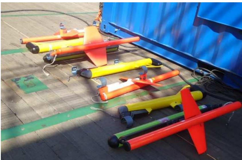
**Fig. 3.4.2.4-1:** DigiBIRD units for depth control and compass navigation (red), recovery system SRD500 (green) and DigiRANGE (yellow)
