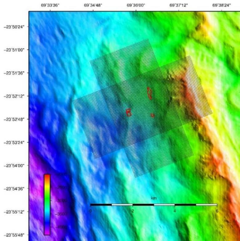
**Fig. 3.1-2:** Planned 3D seismic layout in cluster #4
