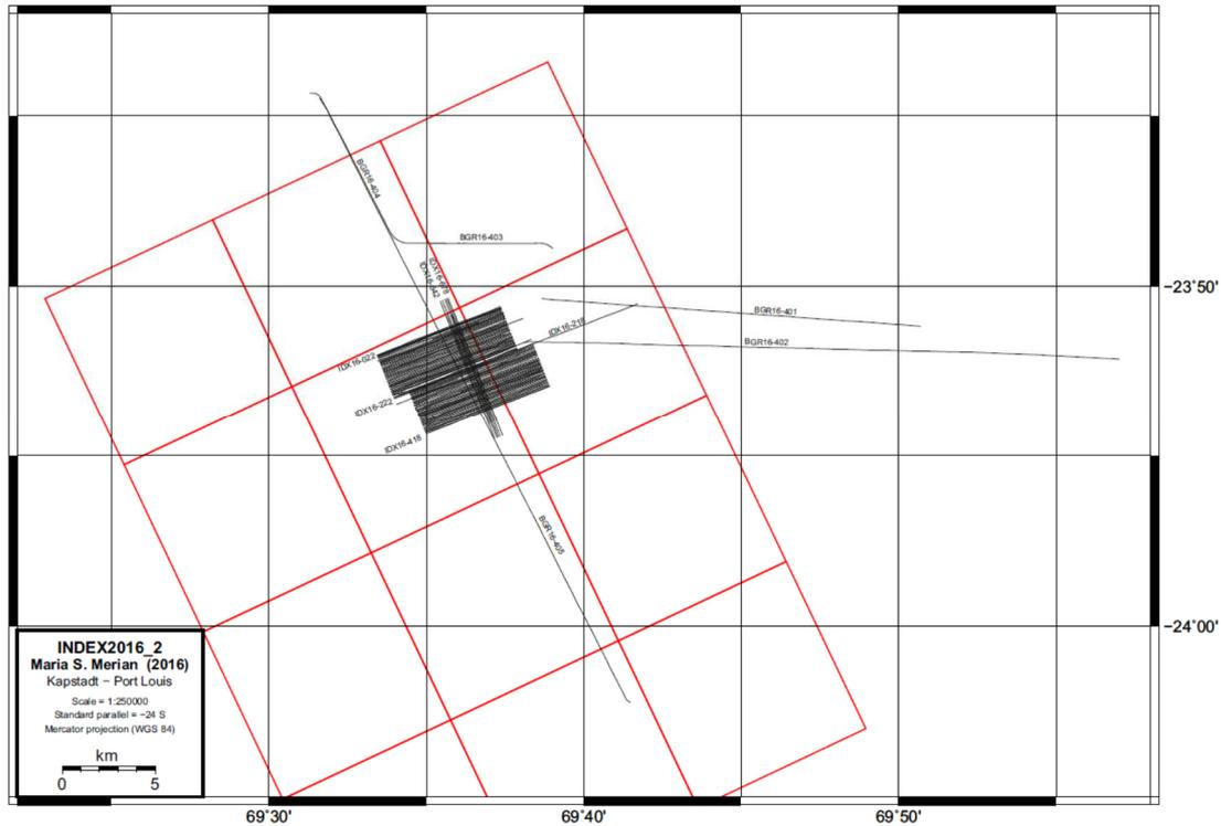
**Fig.3.5-4:** Location of wide-angle seismic lines with respect to the 3D seismic survey area. Red lines mark the individual squares of 10x10 km forming cluster 4 of the license area.
