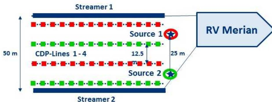
**Fig. 3.4.2.1-1:** Setup of seismic streamers and sources during 3D data acquisition. GI-guns operate in flip-flop-mode (green shots produce green CDP lines, red shots produce red CDP lines).
