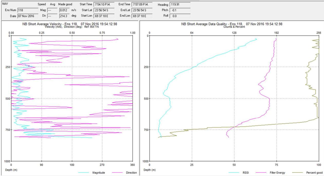
**Fig. 3.4.3.1-2:** ADCP profile in the high frequency range measured on the deployment position of OBS13 (Station 7).
