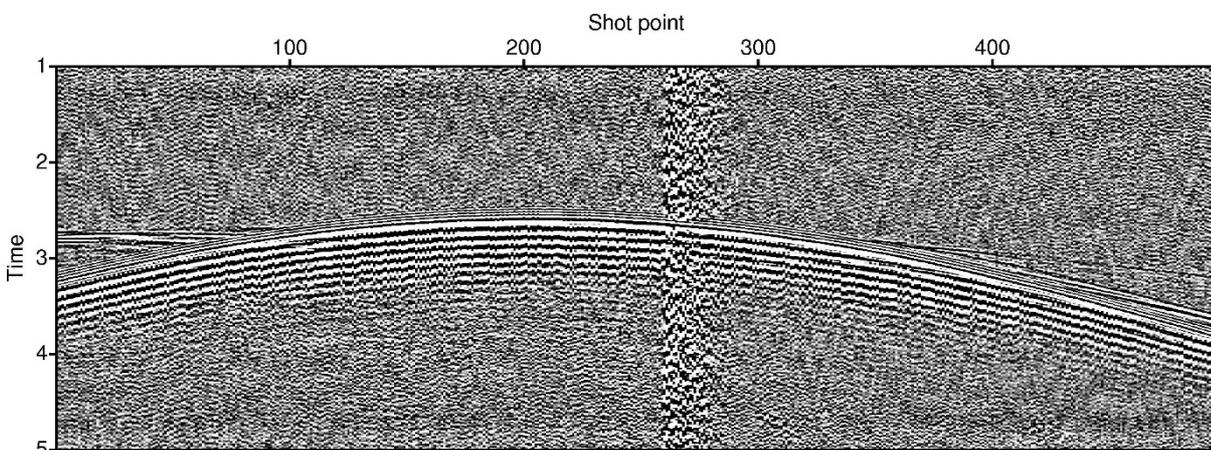
**Fig.3.5-5:** Data example for profile IDX16-034. The whole profile comprises 495 shot points, the first shot point is situated in the east. For OBS 21, the hydrophone channel is shown.
