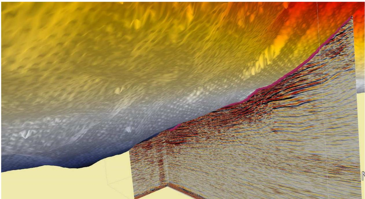
**Fig.3.5-3:** 3D visualisation of a 2D processed inline and crossline seismic profile overlaid with the previously acquired high-resolution bathymetric data of the survey area.
