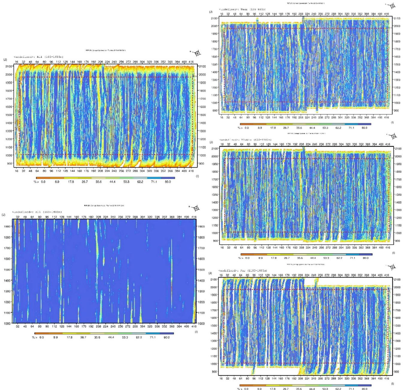
**Fig. 3.4.2-13:** Final coverage of bin cells of the 5 x 6 km cube: All channels before (top left) and after flex binning (bottom left), near channels (top right), mid channels (middle right) and far channels (bottom right).
