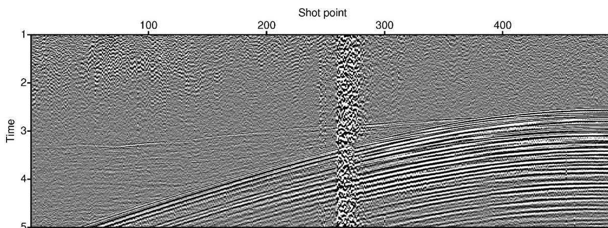
**Fig.3.5-6:** Data examples for profile IDX16-034. For OBS 9 the vertical component is displayed. Both recordings clearly show refracted energy, arriving ahead of the direct wave.
