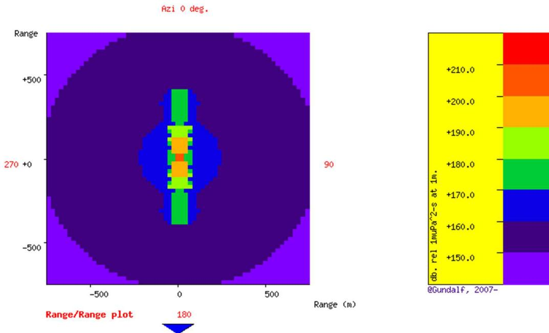
**Fig. 3.4.1-14:** Gundalf modeling of SEL for the single GI-gun. 150 dB re 1  $\mu$ Pa<sup>2</sup>s SEL are expected at a depth of 20 m in a range of 750 m which coincides with our measurements.
