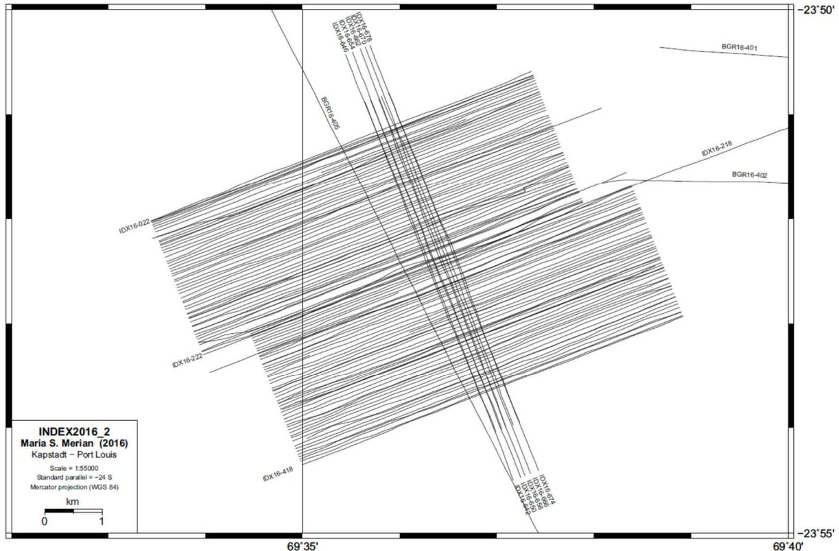
**Fig.3.5-1:** Location of the acquired 115 seismic lines with E-W orientation and 10 seismic lines with N-S orientation
