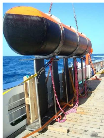
**Fig. 3.4.2.1-4:** Paravane attached to starboard railing
