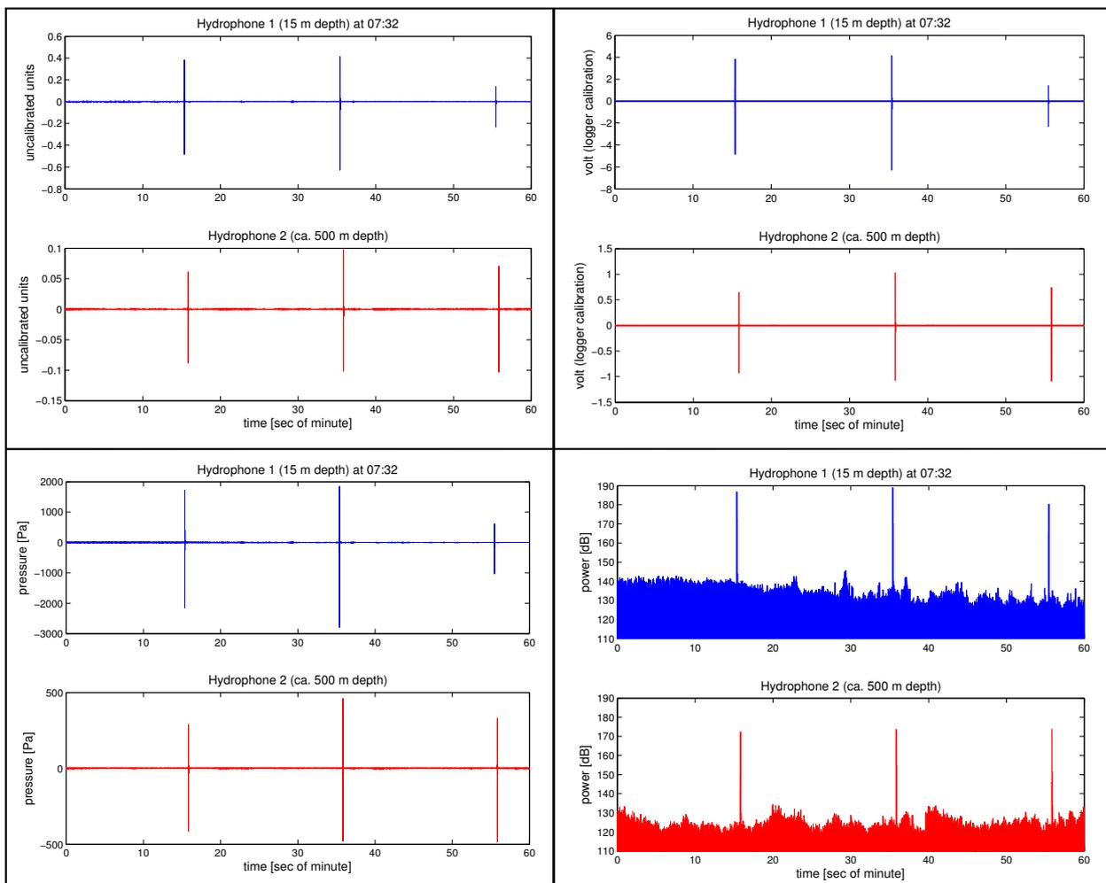
**Fig. 3.4.1-8:** Processing example for one minute (7:32 UTC) including three shots. Raw data in uncalibrated units (upper left panel), volts after applying logger calibration (upper right panel), pressure in Pa after applying hydro-phone sensitivity (lower left panel) and power (or the equivalent pressure amplitudes) in the logarithmic dB scale.
