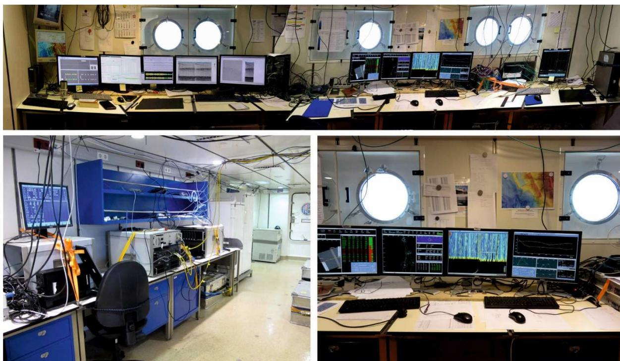
**Fig. 3.4.2-10:** Top panel: Panorama view over the seismic lab monitoring guns, spectra navigation and data acquisition (from right to left). Lower left panel: Spectra RTNU (real time navigation unit), ION System3 Digicourse (streamer birds and acoustics) and Kongsberg RGPS. Lower right panel: spectra navigator's workplace.
