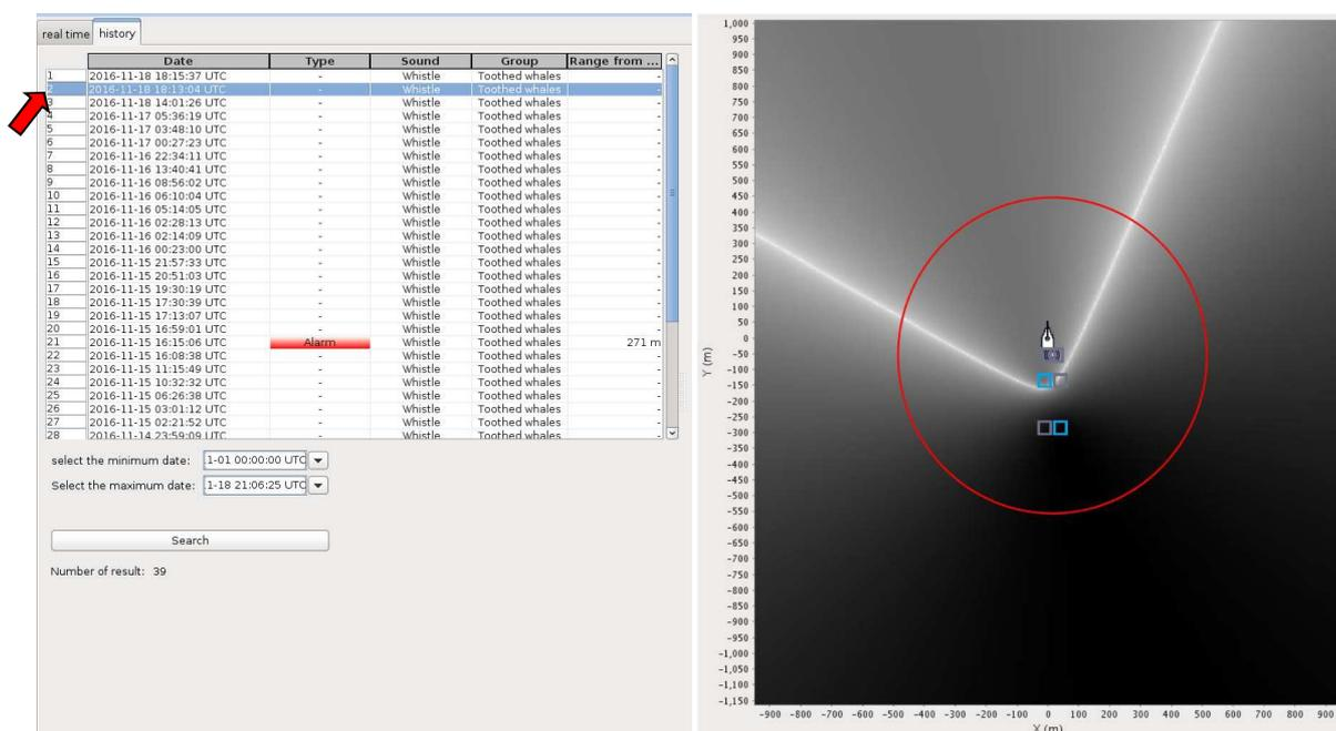
**Fig.3.4.4.-5:** QuietSea detection of the same PAM detection 501 at 18:13 UTC, 18-11-2016 and QS confidence angles of localization (note: event #21, which was categorized as an alarm in the QS history protocol was later identified as a false positive event during post-processing! Verification with PAM recordings still pending.)
