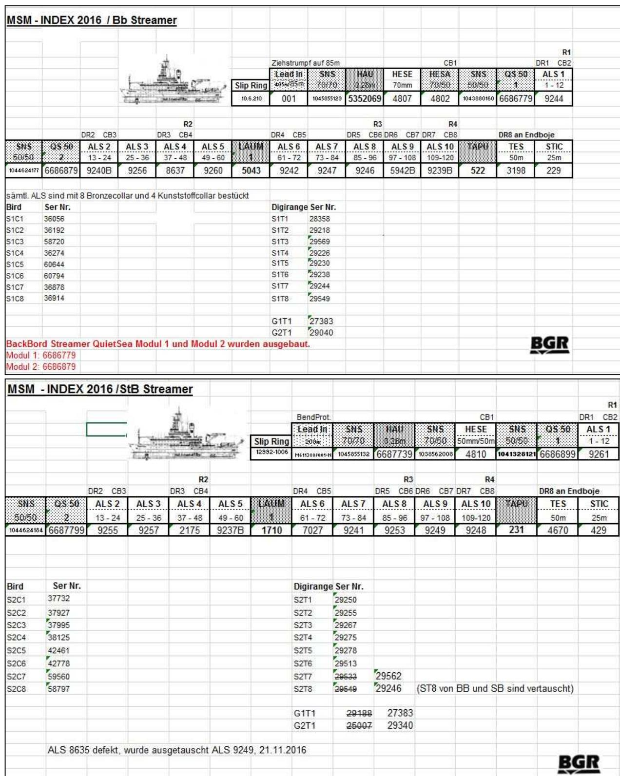
Fig. 3.4.2.4-2a: Streamer configurations for starboard and portside streamers until November-15th
