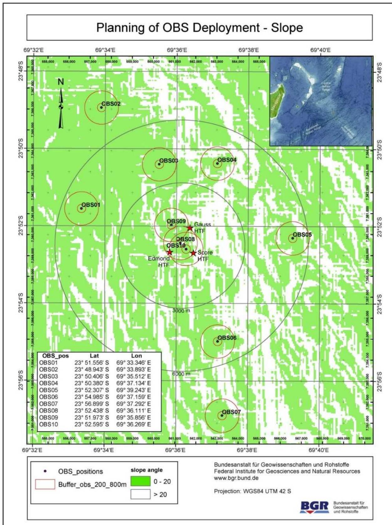
Fig. 3.4.3.1-1: A slope angle less than 20° (green) was a main criterion for the selection of OBS locations.
