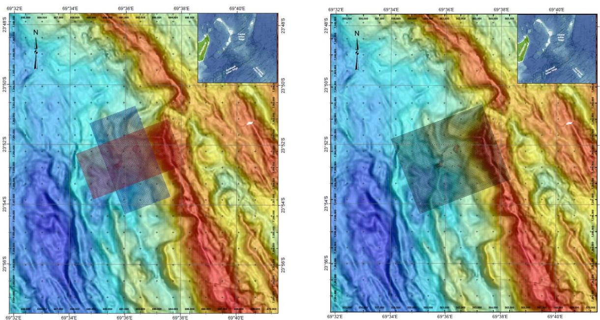
**Fig. 3.4.2-2:** Survey layout for 3D seismic survey as planned originally (left) and modified later (right)
