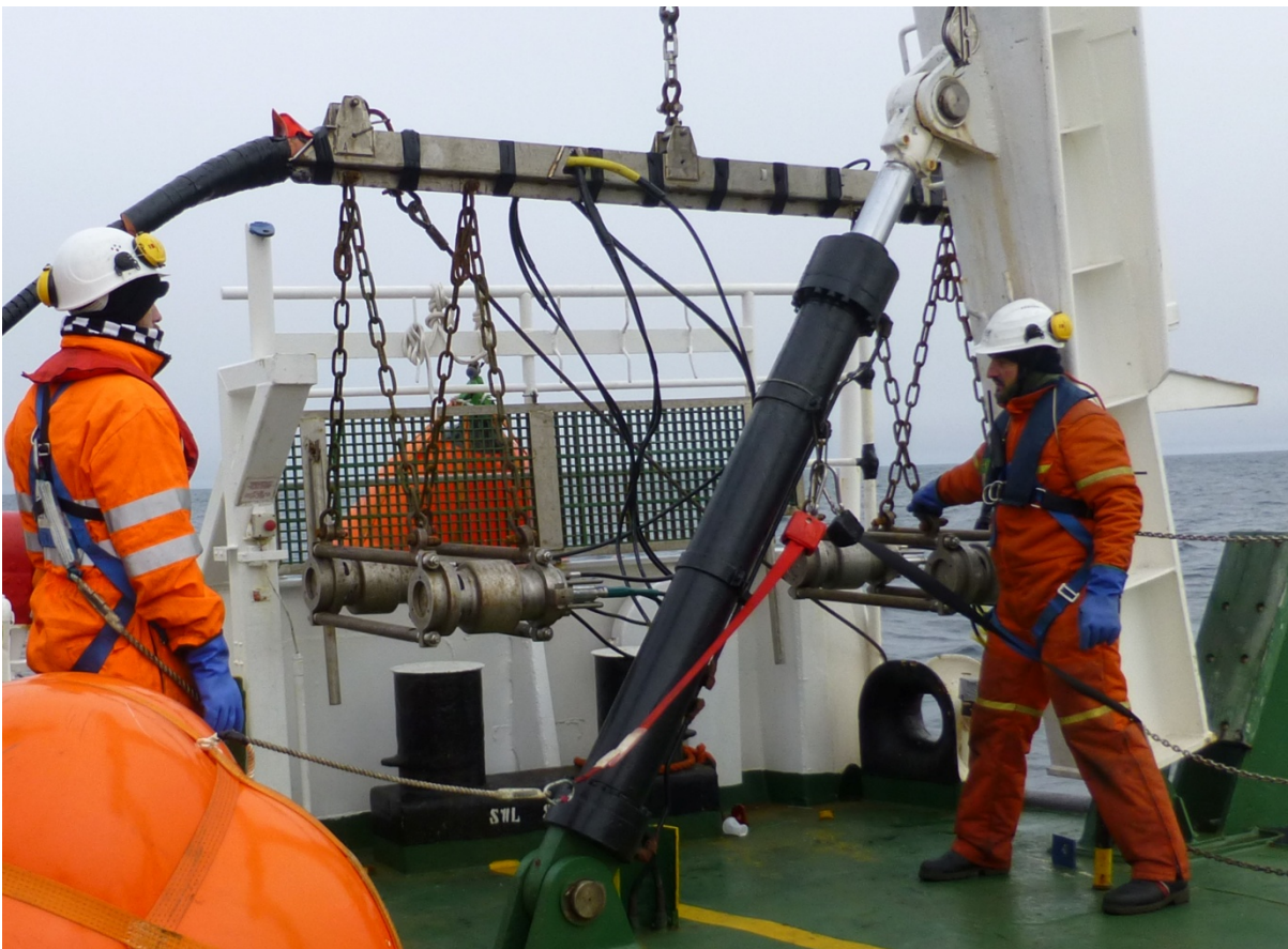
Fig. 33: Starboard G-Gun-Line consisting of two clusters hanging from the A-Frame close before deployment. In background and lower left corner the two buoys (orange) carrying the Gun-Line are to be seen.
