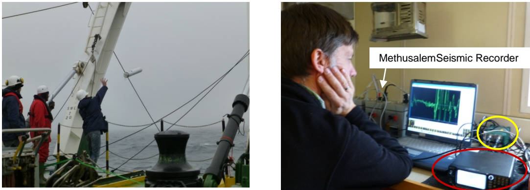
Fig. 37: Launching a sonobuoy from the stern of the vessel – Quality control of the received sonobuoy signal on the bridge deck. Red circle: Yaseo Radio Receiver; Yellow circle: Win-Radio Receiver
