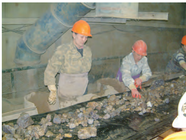
Figure 17: Hand-sorting of fluorite ore in the Bor Ondor plant.
