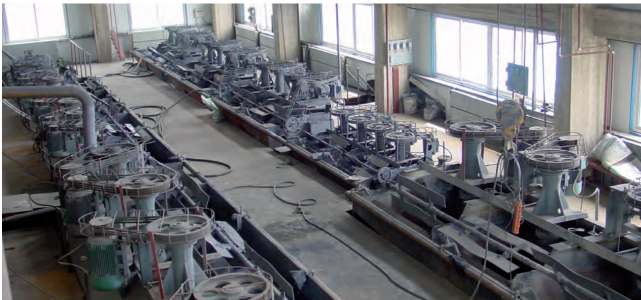
Figure 122: Flotation line as part of the processing facility near Nucht polymetallic deposit.
