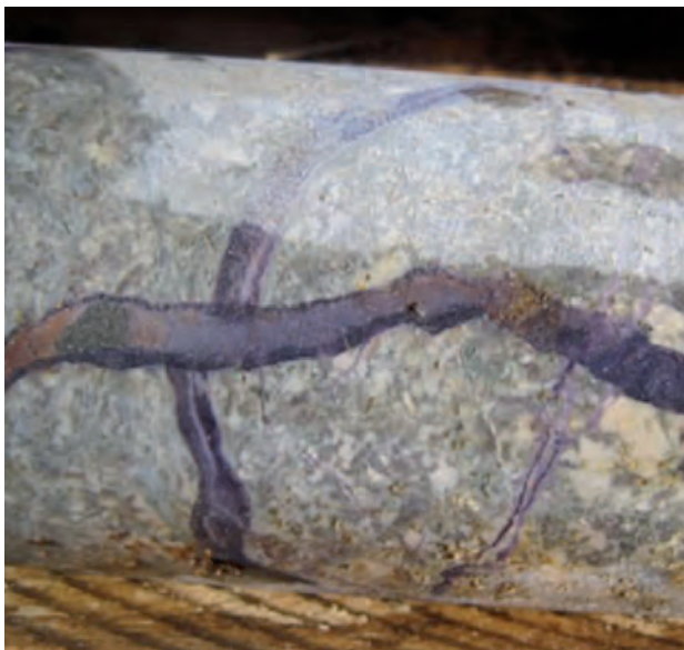
Figure 22: Typical mineralised drill core showing fluorite veining from the Dai Uul fluorite deposit. Photo courtesy of LOTUS RESOURCES PLC.
