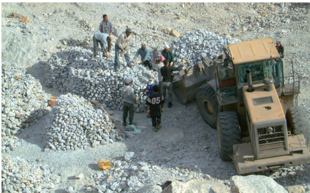
Figure 34: Hand-sorting and loading of high-grade fluorite ore in one of the open pits at Khokh Del (45° 30' 31.5" N, 07° 59' 02.8" E, 1,149 m a msl) as of September 2010.
