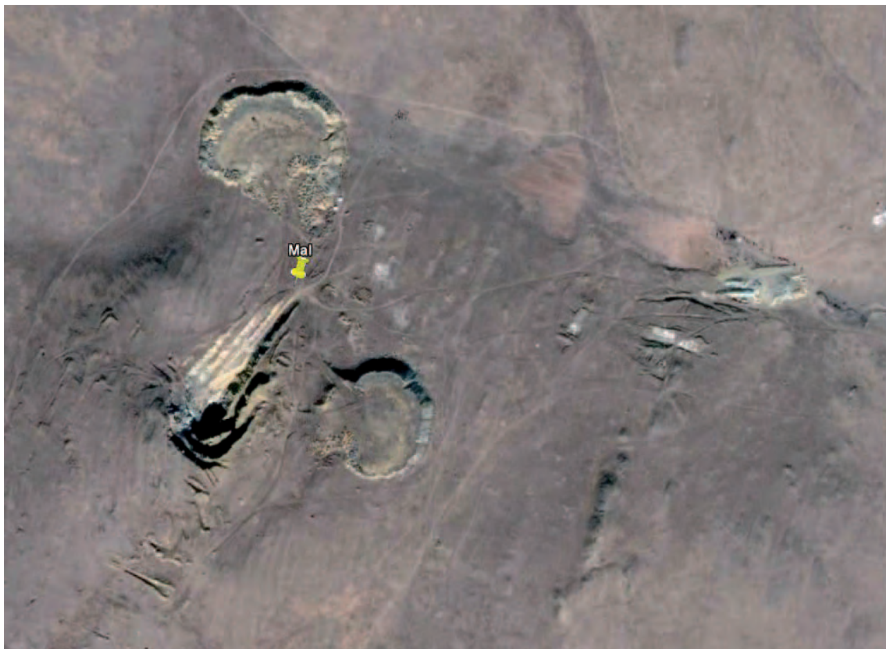
Figure 43: High definition satellite image of the Mal fluorite deposit with an open pit at ore body #2 (Satellite image as of 10 October 2005, Altitude 1.06 km, Photo courtesy of GOOGLE EARTH).
