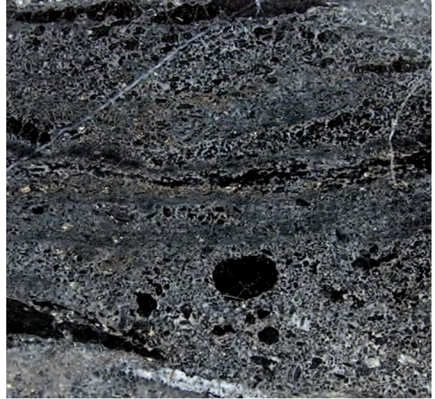
Figure 74: Photo of hand specimen (cut and polished) of typical siliceous breccious ore from the Burenkhaan phosphate deposit. Length shown is 11 cm.
