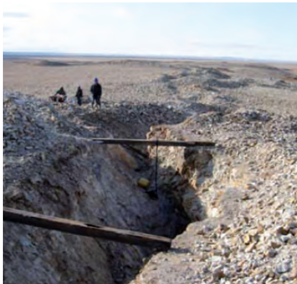
Figure 23: Pilot mining of fluorspar at the Dai Uul fluorite deposit. Under an exploration licence, miners extract high-grade vein type mineralisation using compressor driven jack hammers, buckets, and winches (DORLING 2010a).
