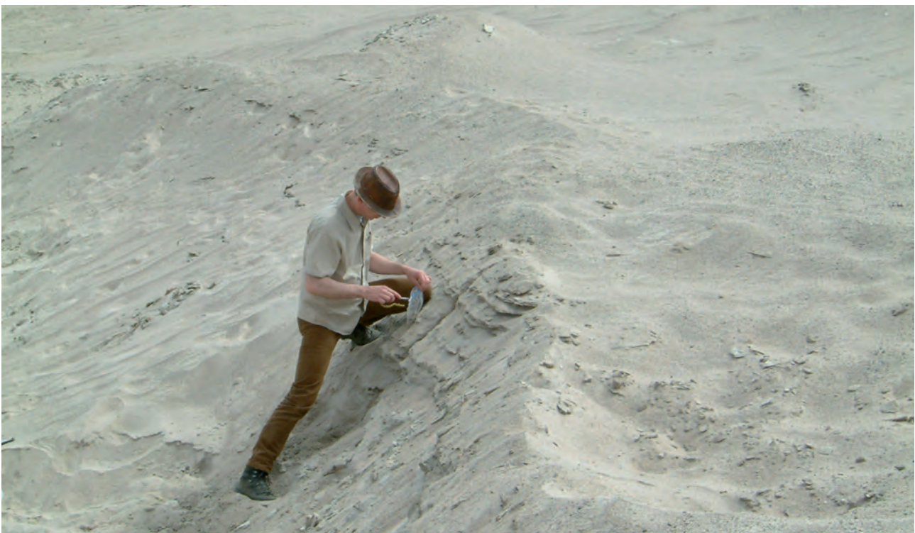
Figure 127: Strip sampling of tailings from the Tsagaan Davaa plant.
