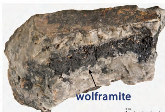
Figure 119: Yeguzer wolframite-molybdenite-beryl deposit: Processing facility of ENGUICAL CO. LTD. (top left), view of the greisen zone (top right), shallow dipping quartz-wolframite vein (bottom left), and high grade wolframite vein type ore (bottom right, scale 5 cm).
