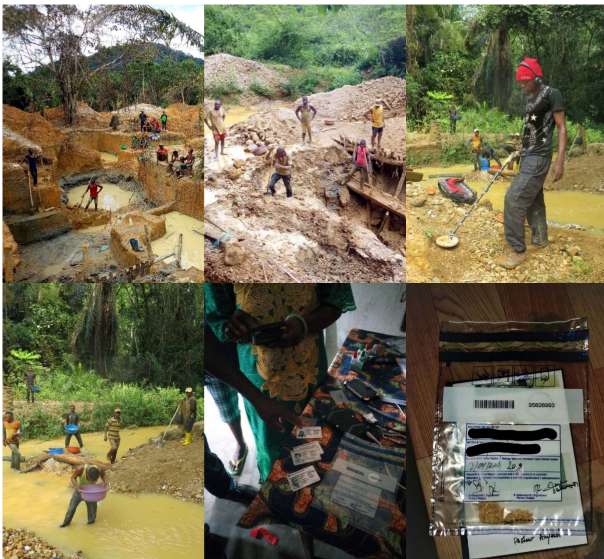
Figure 5: Examples from ASM gold mining at Kampene. Clockwise from upper left: open pit mines in alluvial gold mineralization, detection of gold nuggets using metal detectors, safe gold transport bags (photo credit: ibes AG), registration equipment to facilitate monitoring of gold trade around Kampene, local gold panning.
