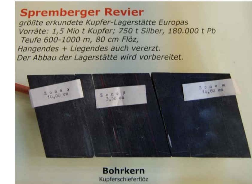
Spremberg Revier Biggest prospected Cu-deposit in Europe reserve: 1,5 mio t, depth: 600-1000 m, 80 cm seam, cheek mineralized too
