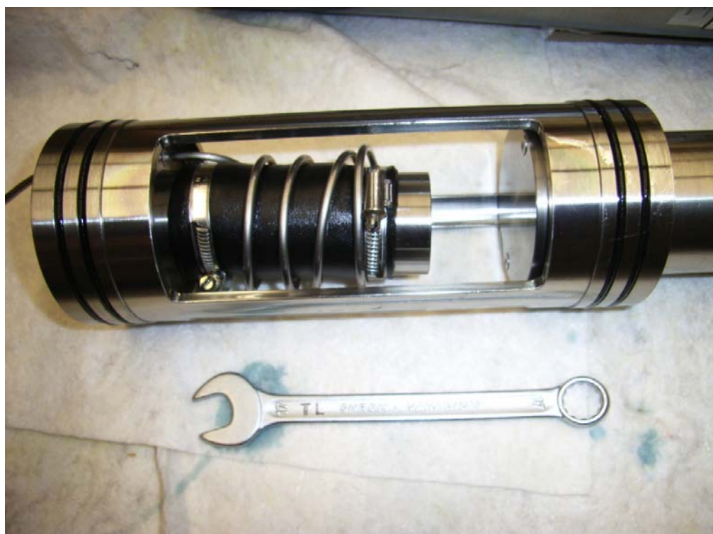
Figure 3.3: Sample holder without (upper figure) and with sample installed (in rubber sleeve, lower figure).
