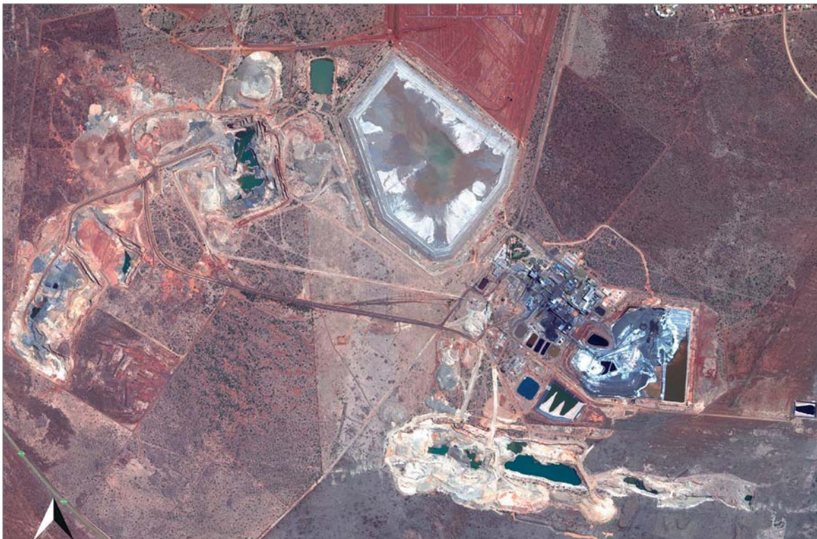
Fig. 3.12: Satellite image of the Rhovan mine area south-west of Bethanie. The active pits are in the western section, while the south-eastern pits are currently inactive (image courtesy of SNL METALS & MINING 2017).
