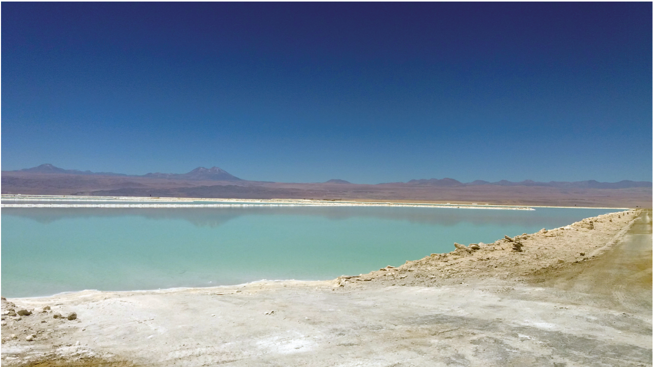
Fig. 6: Evaporation basin for concentrating and purifying Albemarle's lithium-containing brine in the Salar de Atacama, Chile, photo: BGR..
