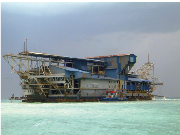
Fig. 9: Floating chain-and-bucket dredger off the Bangka coast. Photo: BGR.
