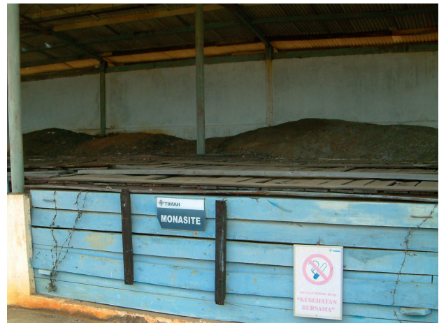
Abb. 11: PT Timah monazite concentrate store. Warnings against possible radiation are absent; however, there is a warning that smoking is harmful, photo BGR.
