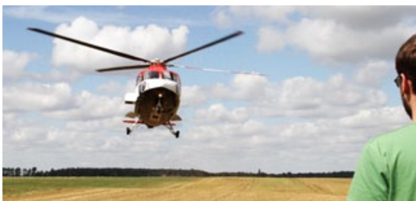
The BGR's Sikorsky S-76B helicopter with the thermal camera equipment on a surveying flight (large and small image).
