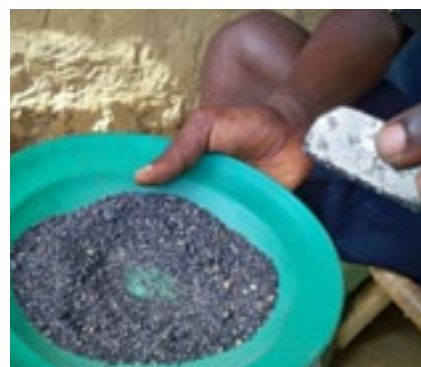
Separating tin ore using magnets, Lulingu, South Kivu province.
