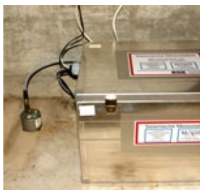
Schematic drawing of mobile station configuration around Insheim: ground movement is registered at the seismometer. The digitiser transmits the data to the BGR data centre in real-time.
