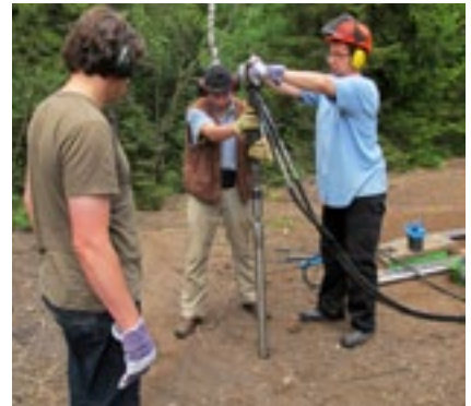
Sampling a mining heap by means of percussion coring.
