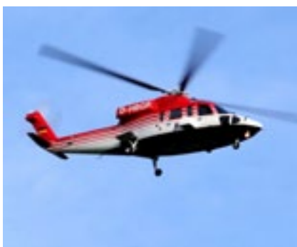
The BGR's Sikorsky S-76B helicopter with the thermal camera equipment on a surveying flight (large and small image).
