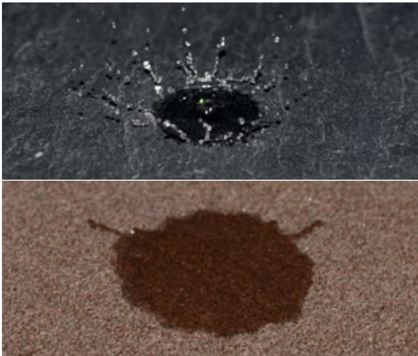
Excellent reservoir rocks (bottom) and barrier rocks effective in the long-term (top) are required for sustainable subsurface storage of CO 2 .
