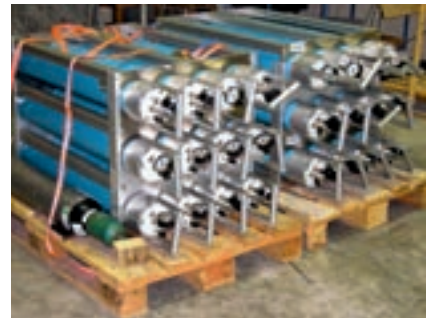
▲ Storage of samples in so-called liners (pressure vessels) in a nitrogen atmosphere.
