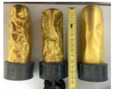
▲ Gold cells can be used to analyse the role of organic sulphur-containing compounds in the formation of gas.
