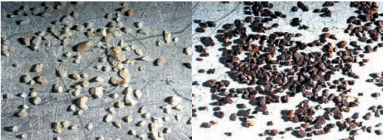
▲ Siderite and ankerite grains (size: 100 – 200 µm) change under the impact of CO 2 and oxygen (left: source material, right: reaction product).
