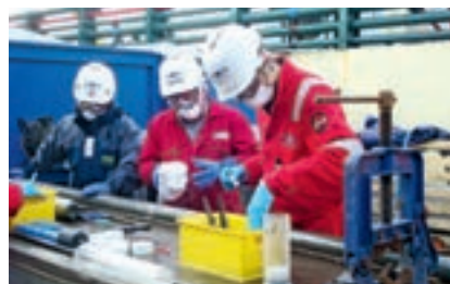
▲ Sampling of a core during IODP expedition 347 – Baltic Sea. During sampling for geomicrobial tests at BGR, the scientists on board Greatship Manisha wear surgical masks and gloves to prevent contamination.
