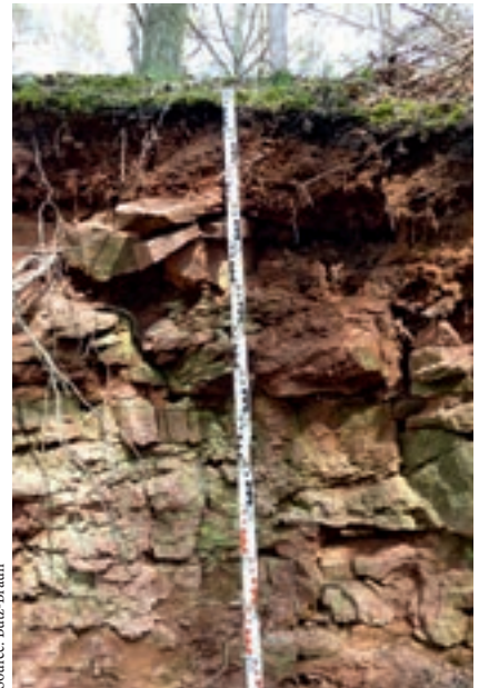
▲ Profile for sampling the weathering properties of the Buntsandstein.
