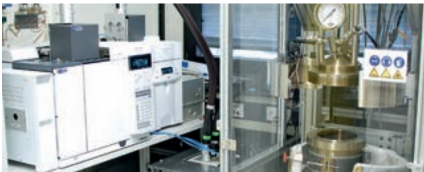
▲ Gas chromatograph (left) to analyse the release of hydrocarbons from source rock under subsurface conditions, directly linked to a high-pressure reactor (right).
