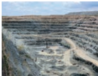
▲ Open-cast mine at the Platreef, South Africa. The weathered platinum ores near the surface are clearly recognisable by their brown colouring.
