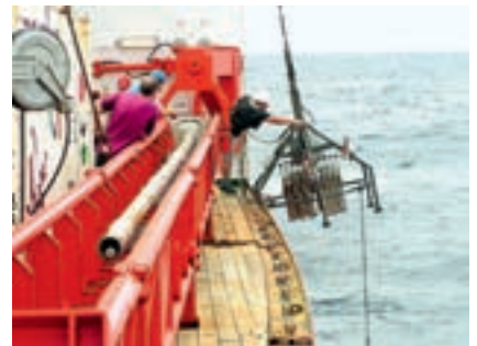
▲ Lowering the box corer from the vessel for use on the seabed.
