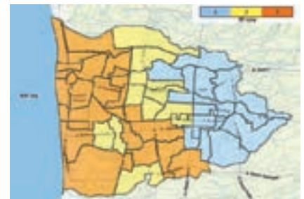
▲ The microzonation map of the city of Mataram shows areas with different levels of seismic hazard (blue=lowest, orange=highest), relative to the city's average level of hazard. The map is based on seismic surveys at about 500 points in the city area.
