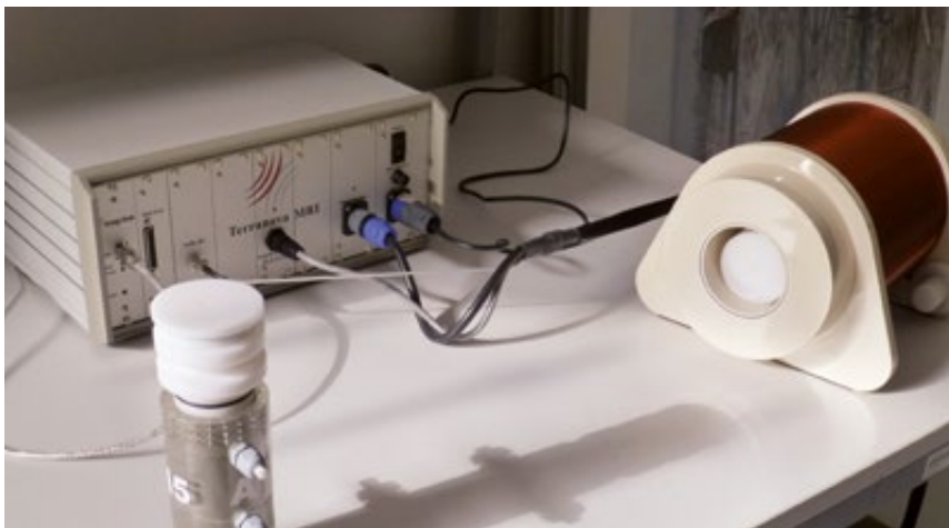
▲ Miniature version of a magnetic spin tomograph for measuring the nuclear magnetic resonance of sediments and soil samples.
