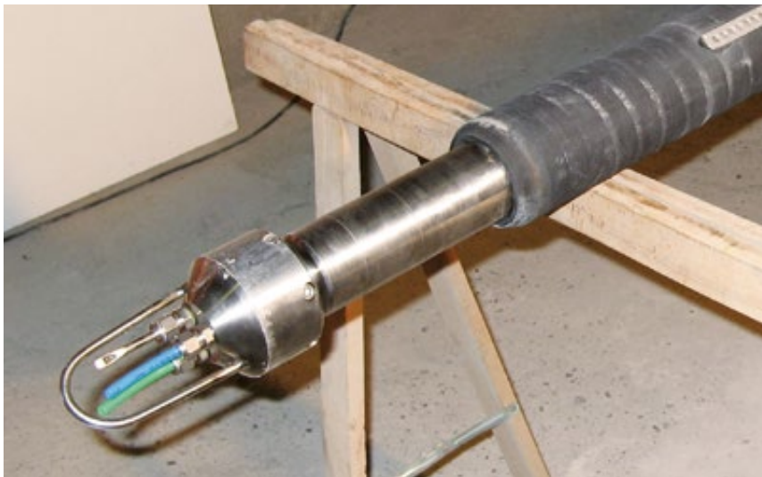
▲ Slot packer to determine the hydraulic anisotropy of the direction-dependent hydraulic properties of the claystone.
