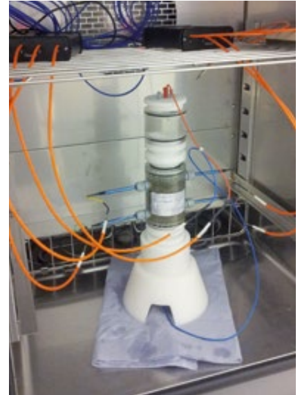
▲ Measuring the electrical impedance of a sediment sample in a climatic cabinet.
