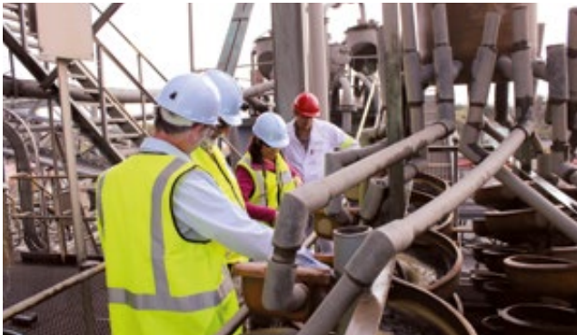
▲ Processing chromites and platinum group metals from tailings material.
