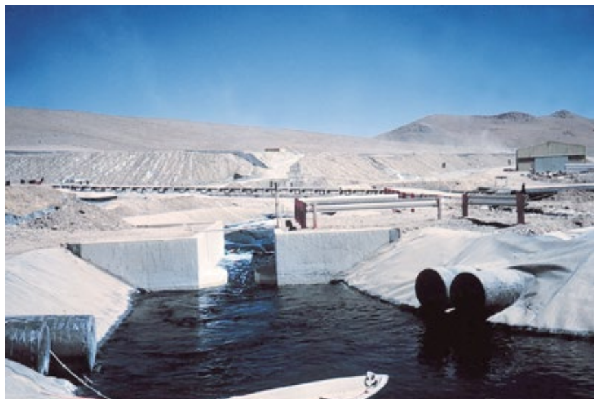
▲ Pregnant leach solution containing copper at a heap bioleaching plant in Chile.
