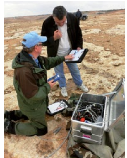
▲ Commissioning a seismic station to record possible aftershocks. The procedure is accompanied by a state representative of the country being inspected.
