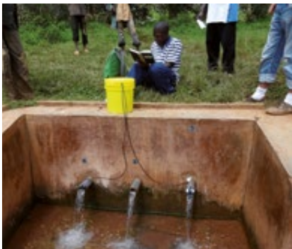
▲ Measuring the conductivity of groundwater during a tracer test.
