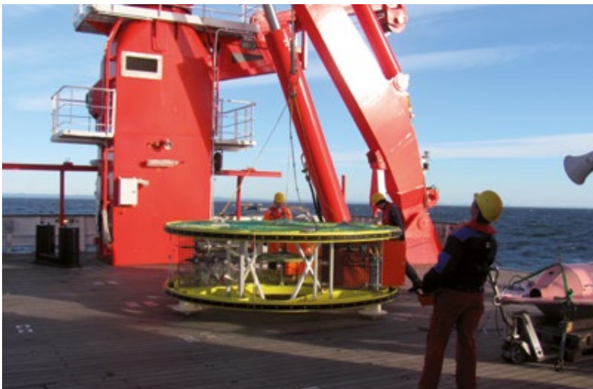
▲ The Golden Eye electromagnetic surveying system was tested for the first time to prepare it for its future deployment in the German massive sulphide license areas.
