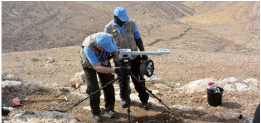
▲ The precise determination of the location of the seismological stations – such as being determined here by two inspectors – is a prerequisite for the subsequent analysis of the ground motion recorded by the instruments, which may hide signs of possible aftershocks.
