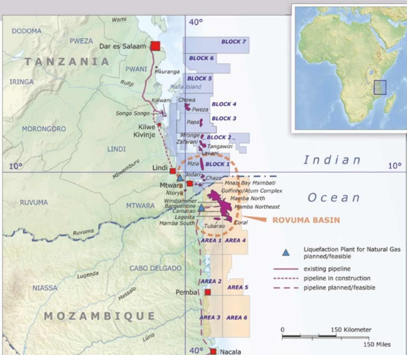
▲ Offshore permit blocks in the Indian Ocean off the coast of Mozambique and Tanzania. Also showing the largest natural gas discoveries, pipelines and liquefied natural gas plants (LNG).
