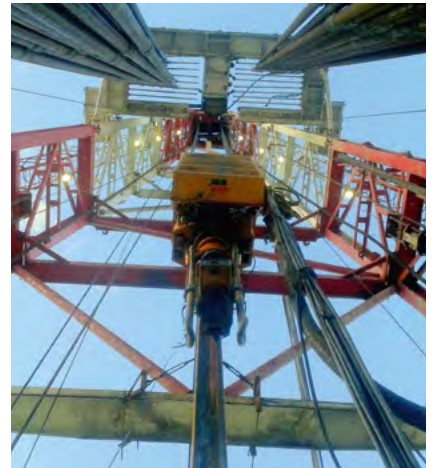
▲ A view from the substructure up into the derrick of a drilling rig with a pulley and hook in the Menengai field in Kenya.
