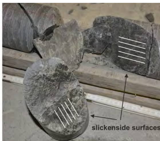
▲ A fault zone in a claystone under the electron microscope (l.) and in a drill core (r.). The slickenside surfaces reveal the direction of the movement.
