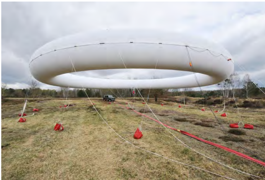
▲ The coil measuring the nuclear magnetic resonance of the groundwater floats over the surveying area with the help of the balloon.
