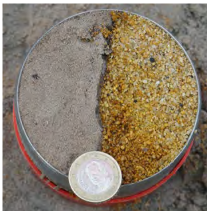
▲ Core sample from the wall of a borehole showing deposits of fine particles.
