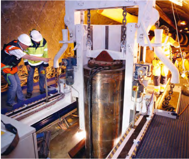
▲ Employees of the Swedish company SKB install the dummy containers for the radioactive waste emplacement test in underground test tunnels in the Swedish Äspö Hard Rock Laboratory.
