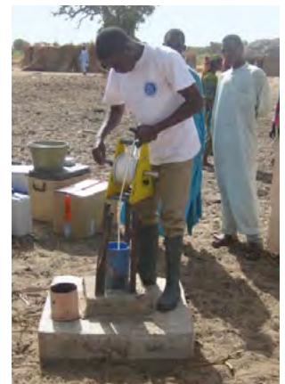
▲ Groundwater level is measured from a monitoring well.
