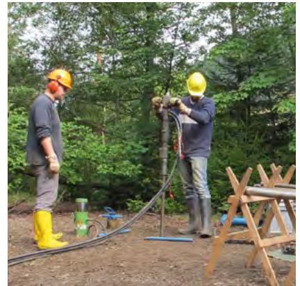
▲ Cores cut by ram core sampling on the Pochsand heap near Clausthal-Zellerfeld in the Harz Mountains.
