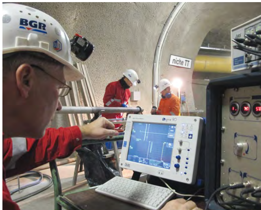
▲ BGR scientists in the Mont Terri Rock Laboratory in Switzerland. They use high resolution geophysical surveying methods to investigate whether claystone is suitable as a host rock for the final disposal of high-level radioactive waste.
