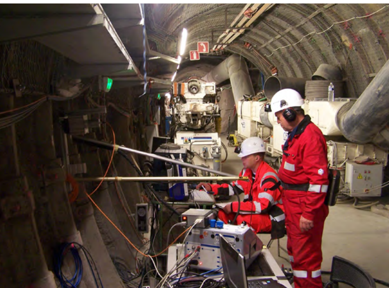
Seismic surveys in clay rocks in an underground research laboratory (France).
