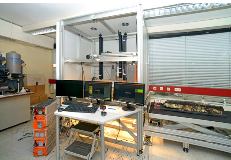
Hyperspectral laboratory scanner SisuROCK for reflection spectroscopy characterisation of rock samples.
