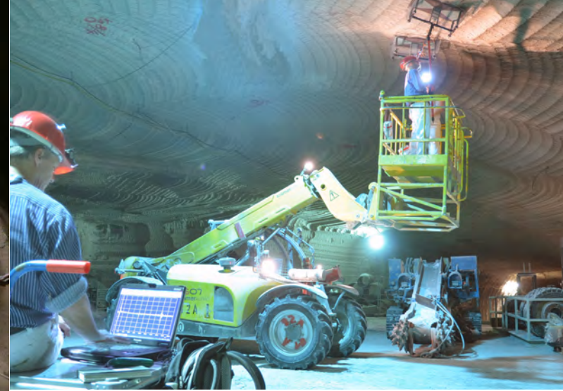
BGR's electromagnetic reflection method for investigating a salt structure.
