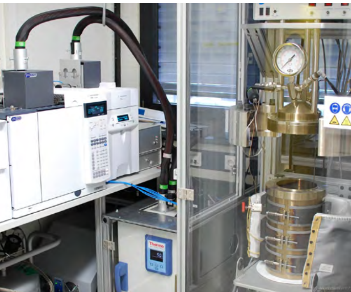
A high-pressure reactor system with online-analysis equipment connected for investigating the conversion of organic matter within rock cores.
