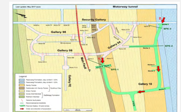
Site map of the Mont Terri rock laboratory with planned 2018 extension (green).
