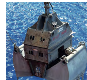
Some of the equipment used by BGR to explore the seabed for sulphide ores (top: Golden Eye. Centre: HOMESIDE. Bottom: TV grab).
