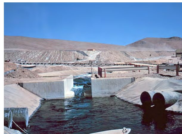
Top: Use of copper heap bioleaching in Chile.
