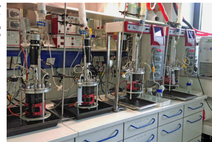
Bioleaching copper in stirred reactors in the BGR geomicrobiology laboratory.
